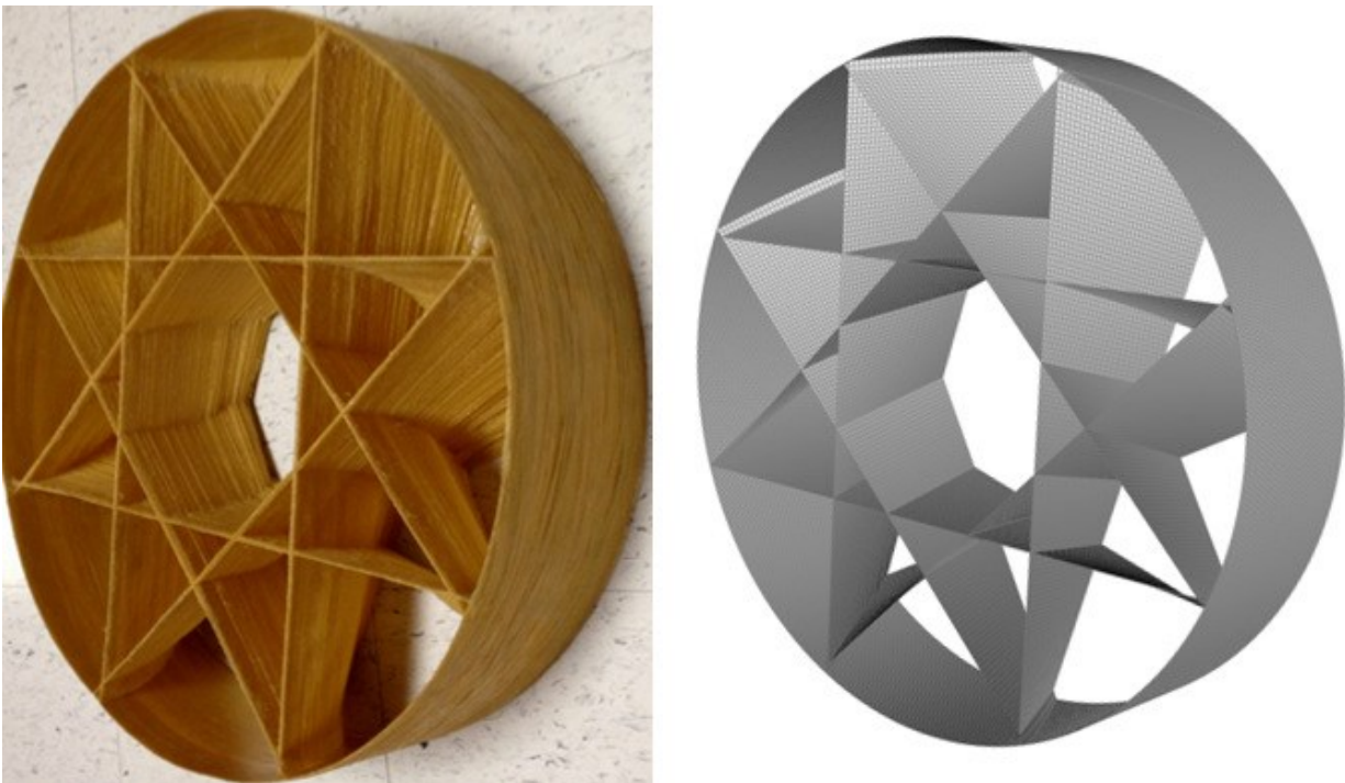
Figure 5.2 Right: Actual woven wheel impeller, Left: Meshed model of the woven wheel in ANSYS ACP
