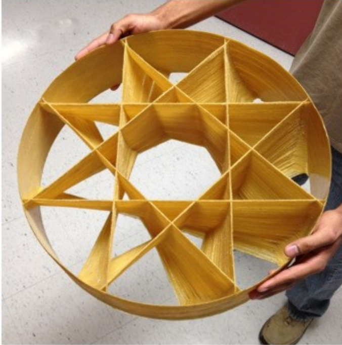
Figure 4.1 Kevlar wound composite impeller with its dimensions
