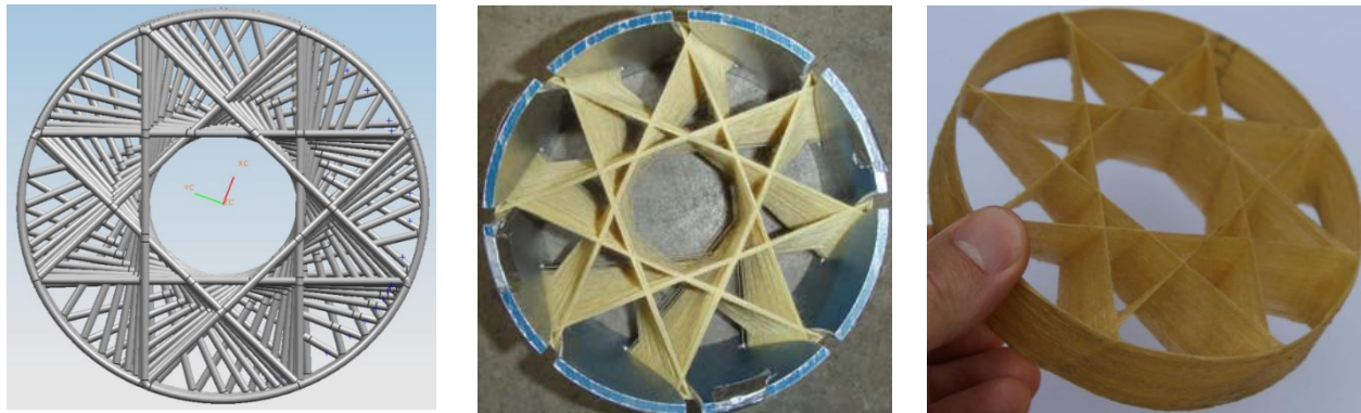
Figure 2.4 (left) Winding pattern computer simulation, (center) wound impeller with mandrel, (right) wound Kevlar impeller
