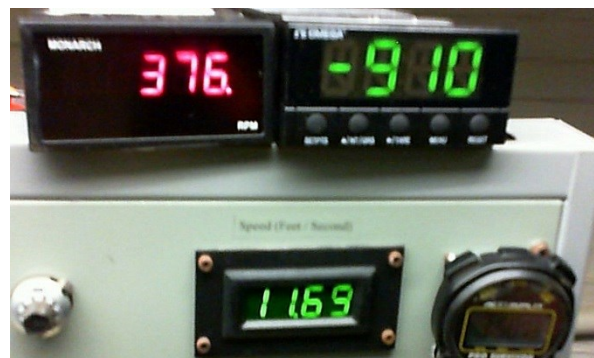
Figure 6.11 Data acquisition for measuring turbine rotational speed, load cell reading and moving carriage speed
