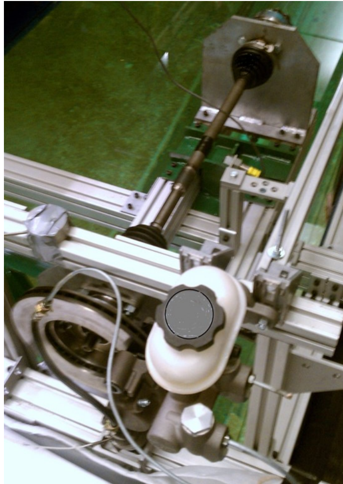
Figure 6.10 Disk brake system with load cell underneath for braking torque measurement
