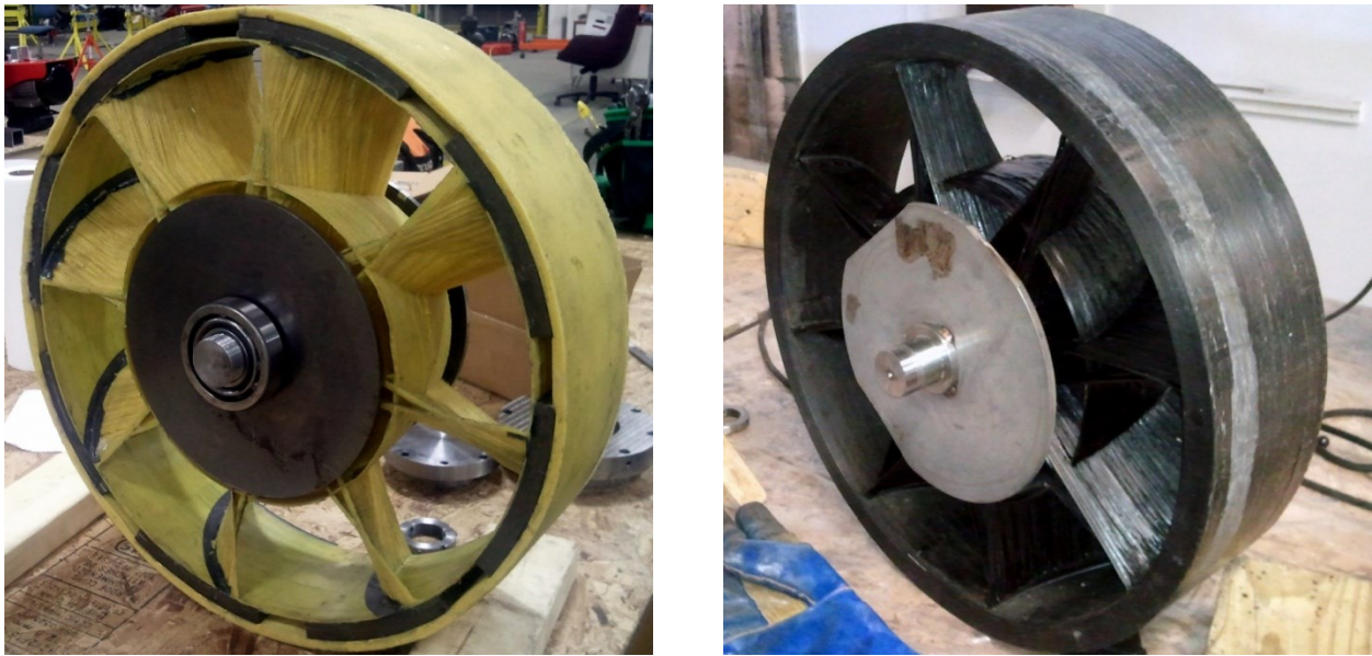
Figure 3.7 Prototype Composite Integrated Impellers (left) Kevlar/epoxy, (right) Carbon/epoxy
