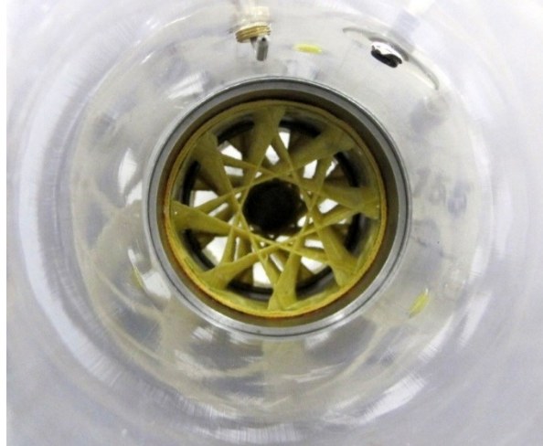
Figure 2.12 Wound Kevlar Wheels as seen from inside the loop
