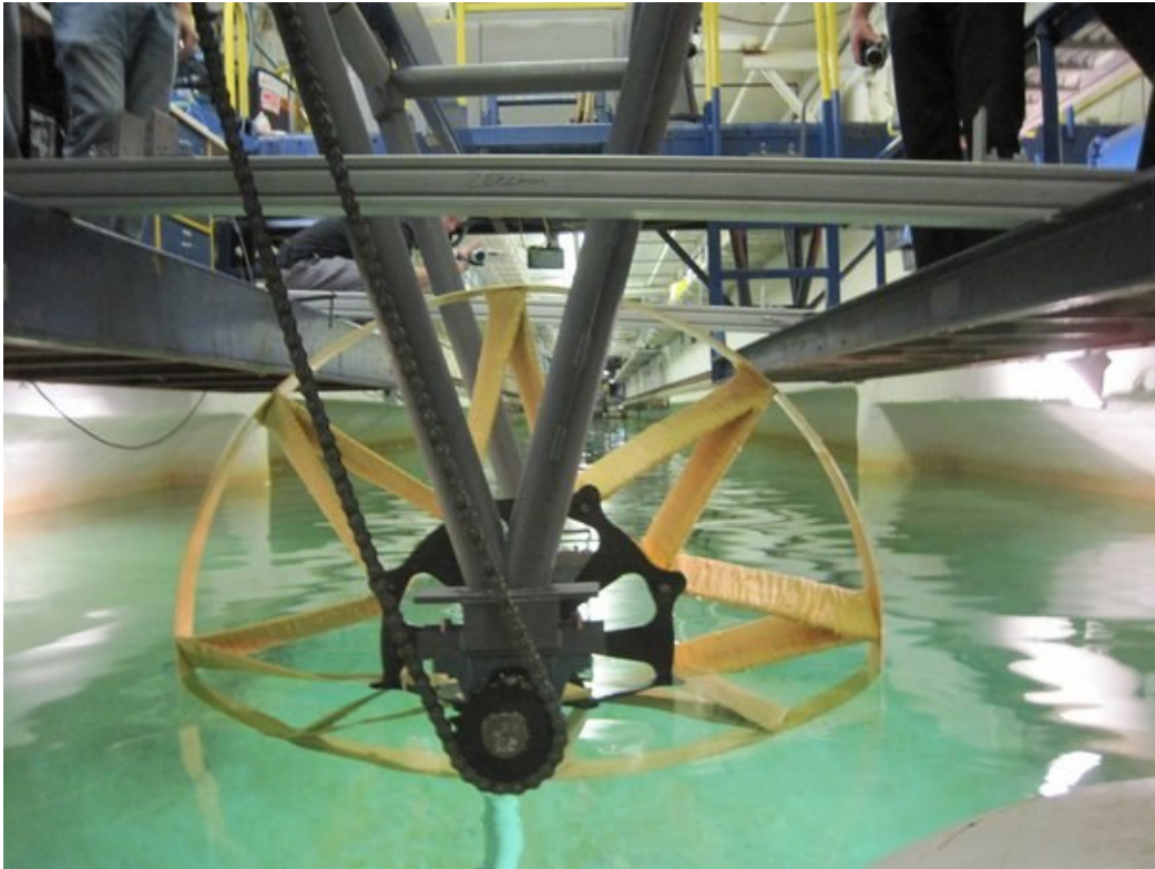
Figure 6.6 Woven wheel turbine with the power transmitting mechanism
