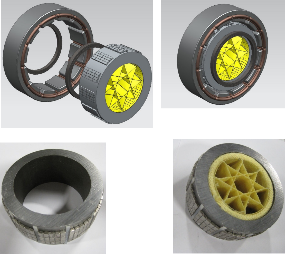
Figure 2.9 Top left: Exploded view of the integrated motor rotor with the composite impeller at the center, Top right: Assembled view of the integrated motor, bearing and the wound wheel Bottom left: Permanent Magnet Poles Integrated with Outer Shroud Bottom right: Fully Integrated with Impeller
