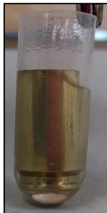
Figure 9. Example of a casing soaking in 700 \mu\text{L} of digestion/tissue lysis buffer.
