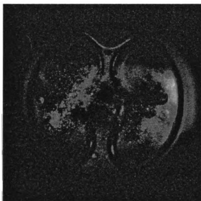
Figure 44. Mie Scattering of Direct Injection at 320° After Top Dead Center Intake, Start Of Injection 240° After Top Dead Center, Fuel Pressure 1000 psi
