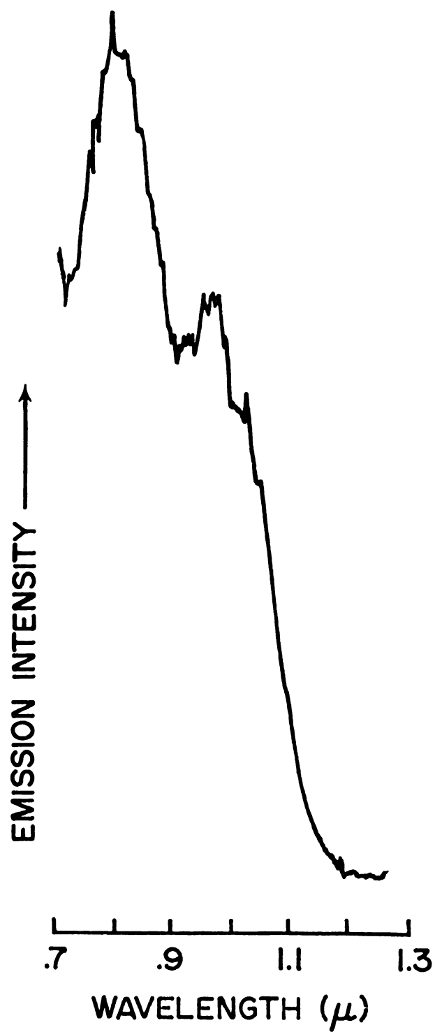
Figure 23. A low resolution chemiluminescence emission spectrum of the near-infrared 0.7 to 1.3 \mu region
