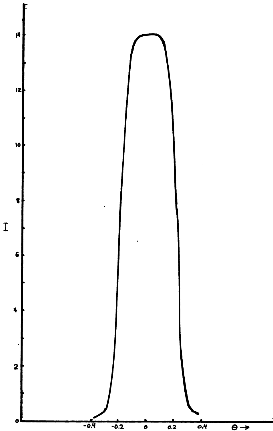
Fig. 47 Single aperture illuminated in the broad source mode. Source of angular breadth \alpha = 2.8 \lambda/D . \theta is expressed in 10^{-3} radians.
