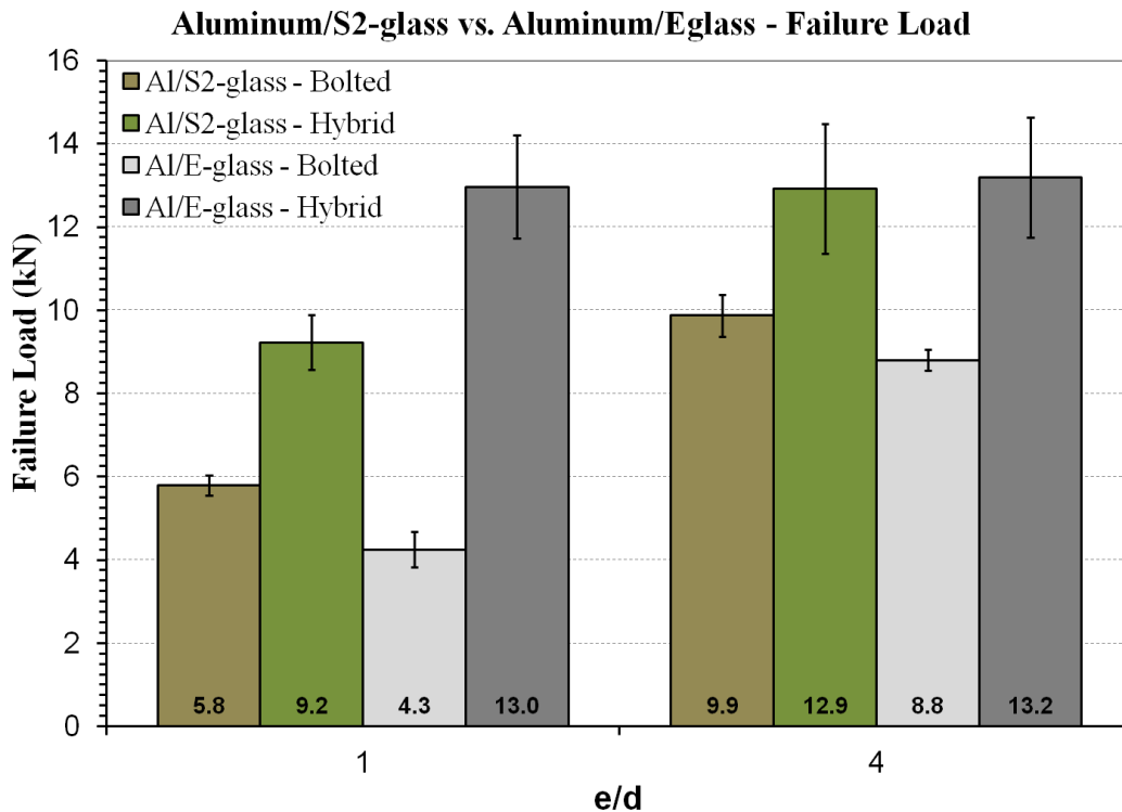
Figure 50: Failure loads of Aluminum/S2-glass and Aluminum/E-glass bolted and hybrid joints, e/d=1 and 4, under impact loading.
