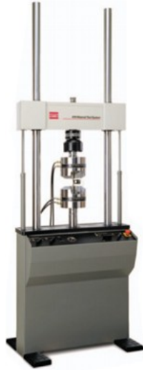
Figure 25: MTS 810 Material Testing System used for static testing at 1 mm/min crosshead displacement.
