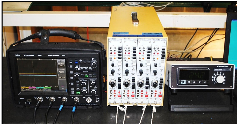
Figure 18: SHTB data acquisition system including 4-channel Lecroy WaveJet 354A digital oscilloscope, Vishay 2310B signal conditioning amplifiers (4), and 10-channel Omega MDSSi8 benchtop indicator (left to right).
