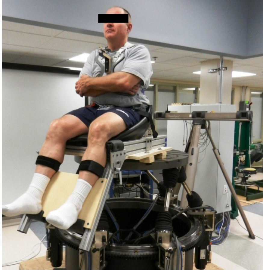
Figure 3.2 Example setup for seated balance testing using the Mikrolar R-3000 Rotopod.
