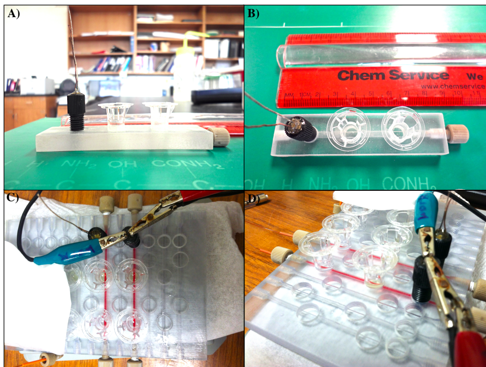
Figure 3.19 Scaling up the original \text{O}_2 and RBC ATP measurement device. The device shown in Figure 3.2 was printed as an array of channels as shown in panels C and D, each with detection wells for NO and ATP and threaded ports for oxygen detection. Alternative views of the original device are displayed in panels A and B.
