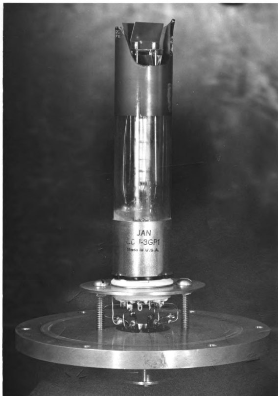
Figure 5. Electron Gun Mounted on Endplate
