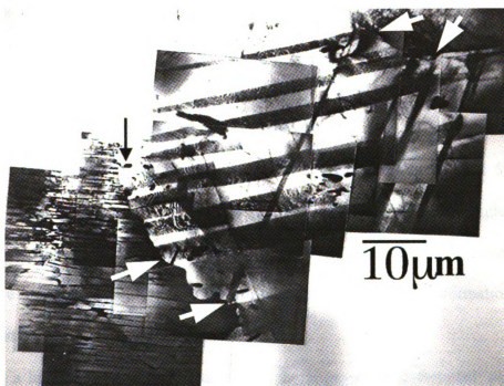
Figure 8.9 TEM image of lamellar and equiaxed grains from the specimen tested at 760°C, 138 MPa (1010 °C/50 hours heat treatment).
