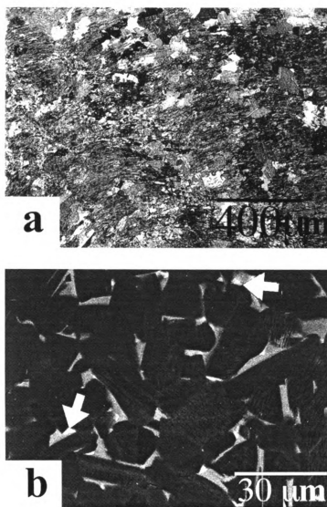
Figure 10.5 Microstructures of As HIPed 47-2-2 (a) optical micrographs before creep test (b) BSE images after creep test.
