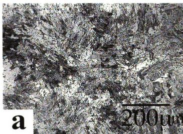
Figure 10.4 (a) optical micrographs of As HIPed 47Al XD before creep test.
