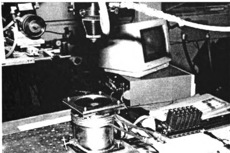
Figure 14. A photograph showing the laser nozzle, the chamber, and the temperature measuring setup.
