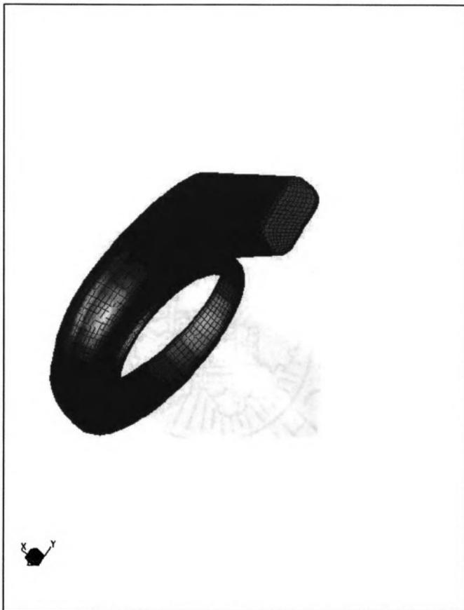
**Figure 6.1: Multi-block Twin Flow Turbine Mesh**
