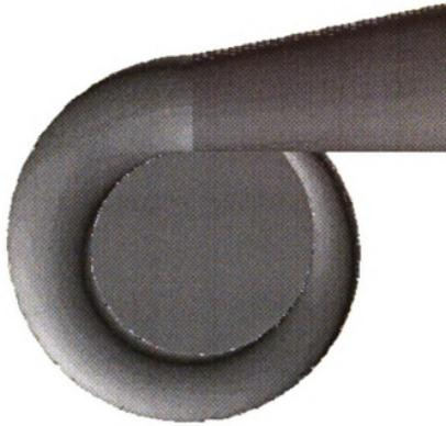
Figure 4.18: Solid model for sample compressor design
