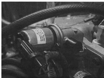
Fig. C.13: Idle Air Control Valve
