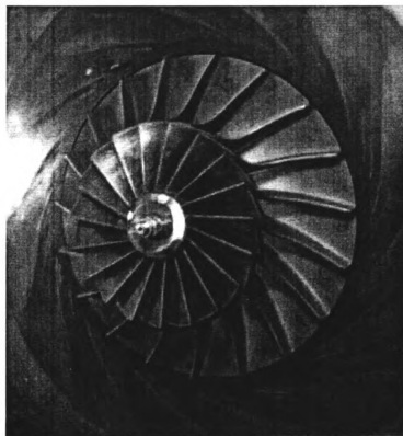
Figure 4.2 Impeller of the tested configuration
