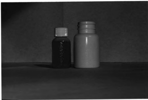
Figure 7: The Difference in Bubbles between HDPE-1 (left) & HDPE-2 (right)
