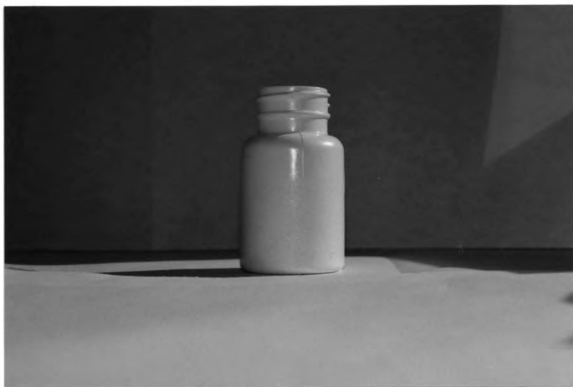
Figure 10: Bubbling of HDPE-2 in the Pure Soy Methyl Ester Test
