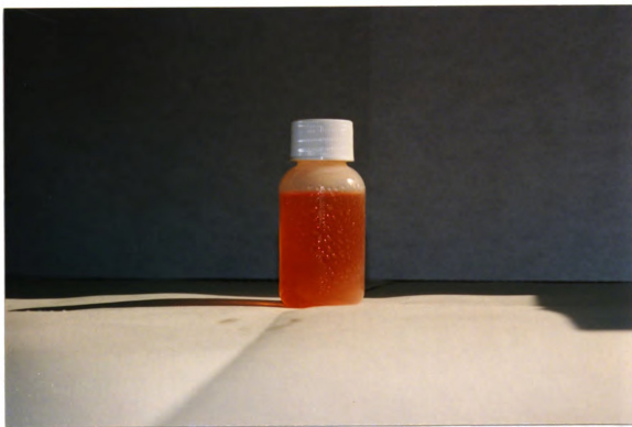
Figure 5: Bubbling of LDPE in the Bean-e-doo Test
