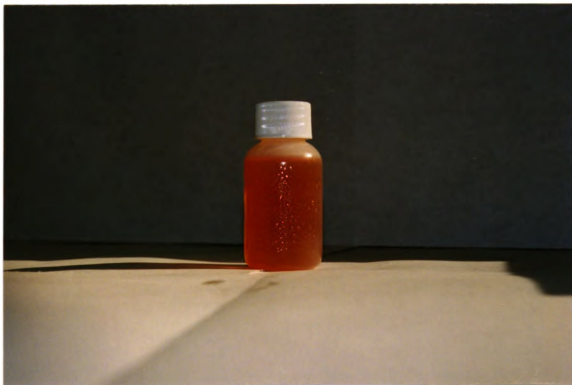
Figure 8: Bubbling of HDPE-1 in the Bean-e-doo Test
