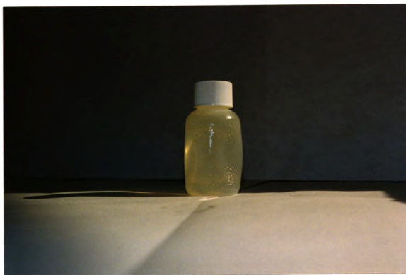
Figure 9: Bubbling of HDPE-1 in the Pure Soy Methyl Ester Test
