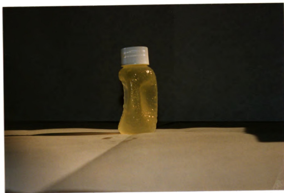
Figure 6: Bubbling of LDPE in the Pure Soy Methyl Ester Test
