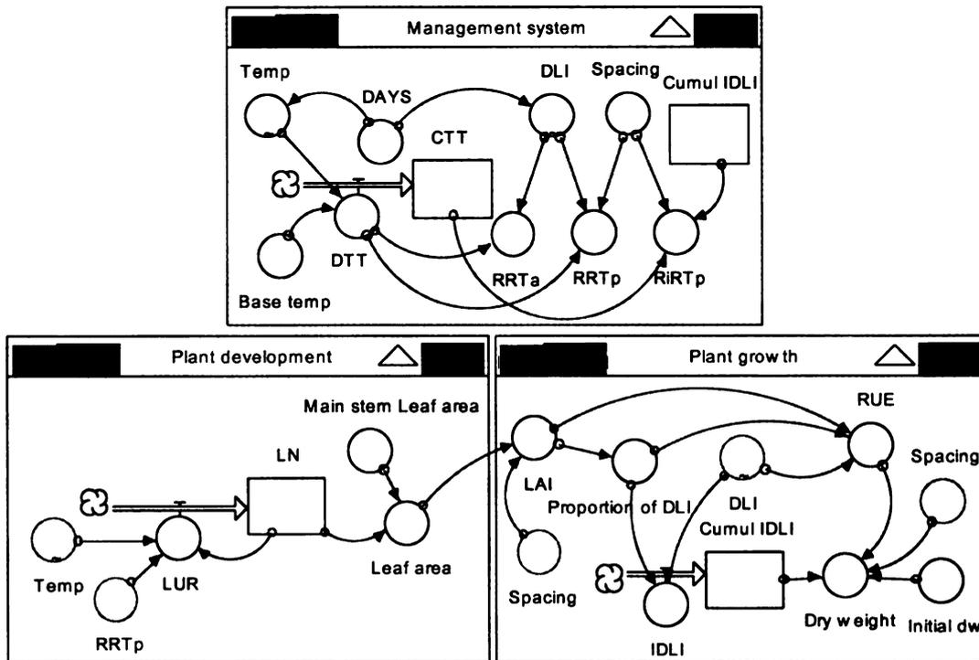
Fig. 2. A STELLA diagram showing the operation of the poinsettia growth and development model. Abbreviations are as described in the text.
