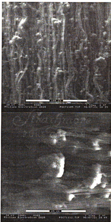
Figure 17 - SEM picture of EPE:PSC(30GLY) E140C, I120C. Tensile fracture zone. Slightly better adhesion. Distribution is uneven and there is room for improvement.
