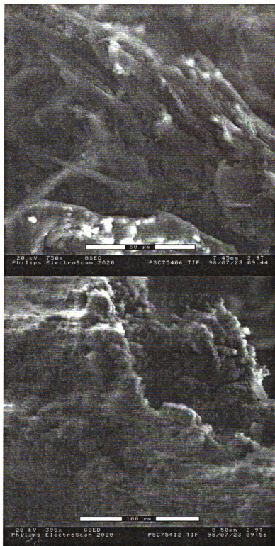
Figure 20 - SEM picture of EPE:PSC(G)::70:30 E135C I135C. Clusters or particles and a very non-uniform distribution of matrix are seen.
