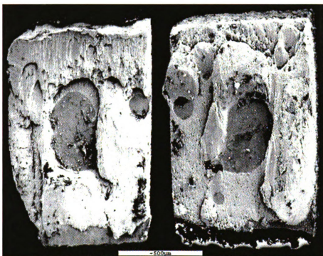
Figure 26b. Non-Composite Fracture Surface, T = 25^{\circ}\text{C} , \tau = 23.5 \text{ MPa} . (Sample 040).
