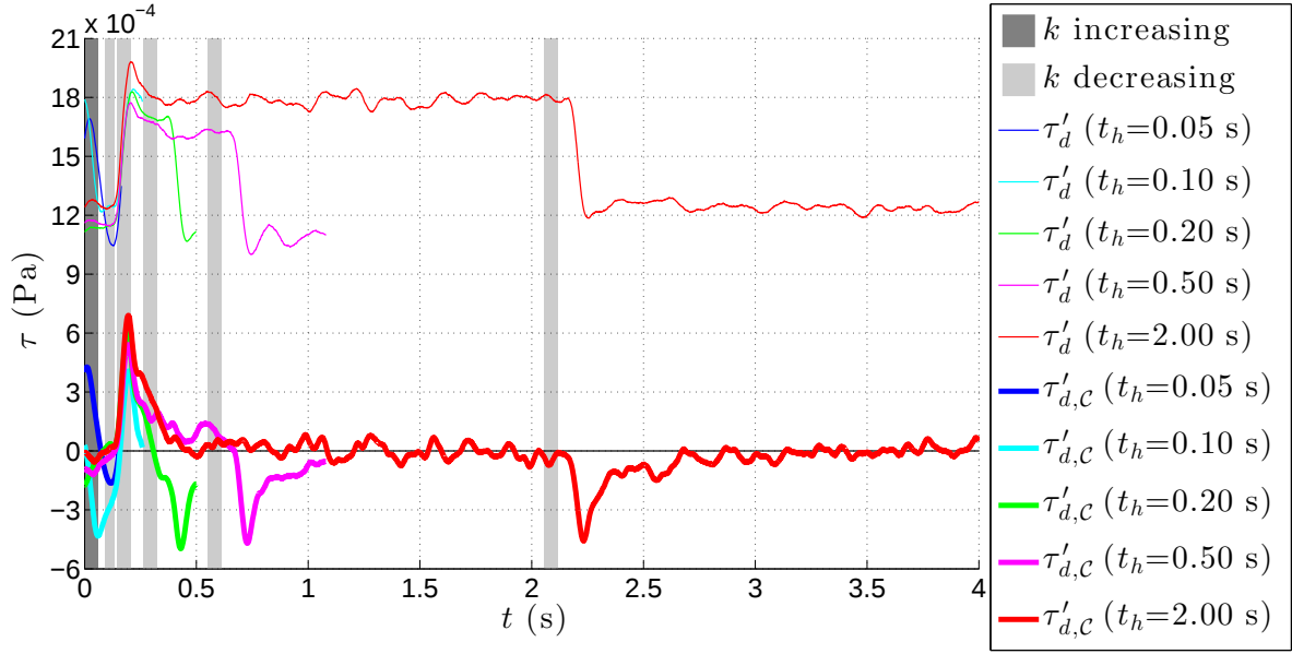
Figure 6.25: Control results with the unsteady roughness element motion from k=1.0 to 1.2 mm with various steady-state hold times, t_h . The uncontrolled results are represented with thin lines, while the controlled disturbance are represented with thicker lines of the same color.
