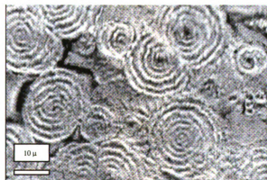
Figure 46. Micrograph of polymer (C_8\pi C_8EO_7)_n under non-crosspolarized light
