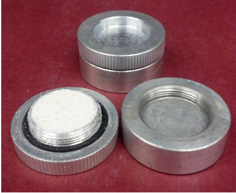
Figure 11. Test cell filled with wheat flour that was used in thermal inactivation studies.
