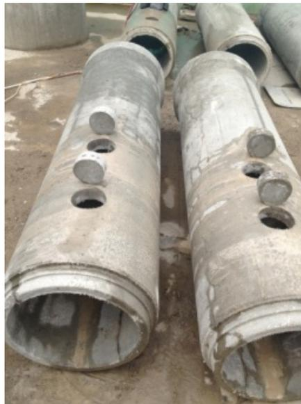
*Figure 13.3 Sorption test specimens cored from pipes.*
