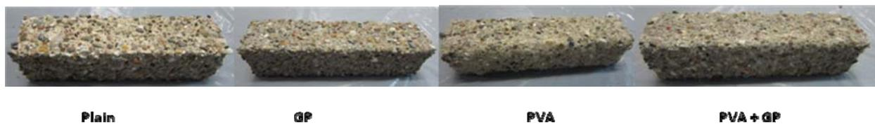
*Figure 13.21 Visual appearance of concrete specimens with different reinforcement systems after 90 Days of acid attack*
