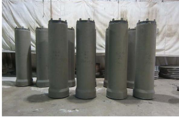
*Figure 13.1 Pipes manufactured with different nano- and/or micro-scale discrete reinforcement systems.*
