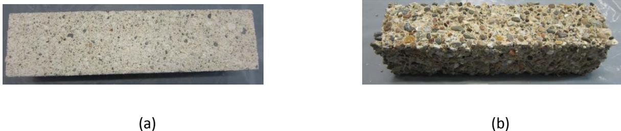
*Figure 13.20 Typical plain concrete prismatic specimens prior to (a) and after (b) 90 days of exposure to acid attack.*
