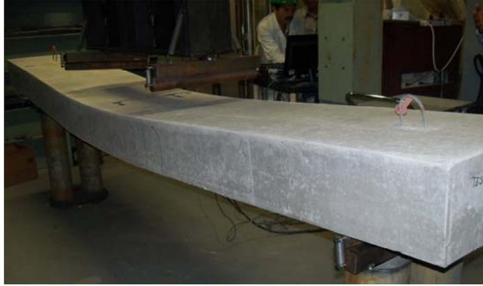
Figure 13.26 An example reinforced concrete beam after flexural failure.
