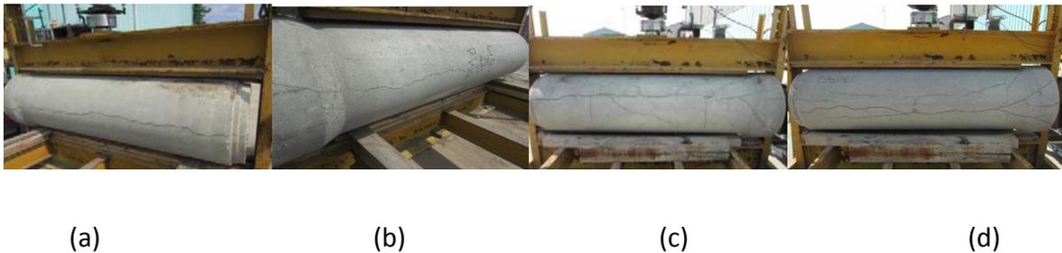
*Figure 13.7 Crack propagation patterns for (a) control pipe; (b) pipe with PVA fiber; (c) pipe with nanoplatelet; and (d) pipe with nanoplatelet and PVA fiber reinforcement.*
