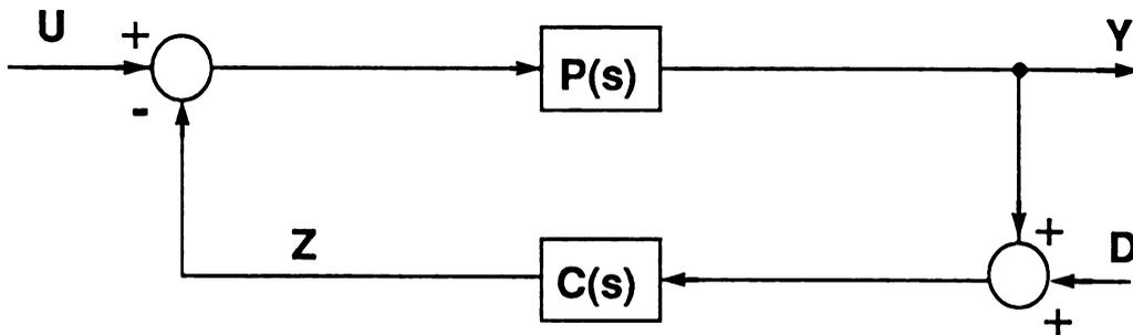
Figure 2.1: The feedback control system including measurement noise
