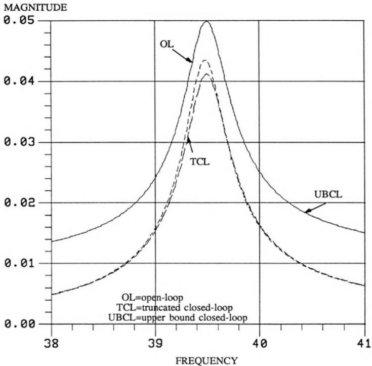
Figure 5.7: Detailed closed-loop frequency response of the 2nd mode
