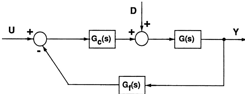
Figure 4.1: The feedback control system including input disturbances
