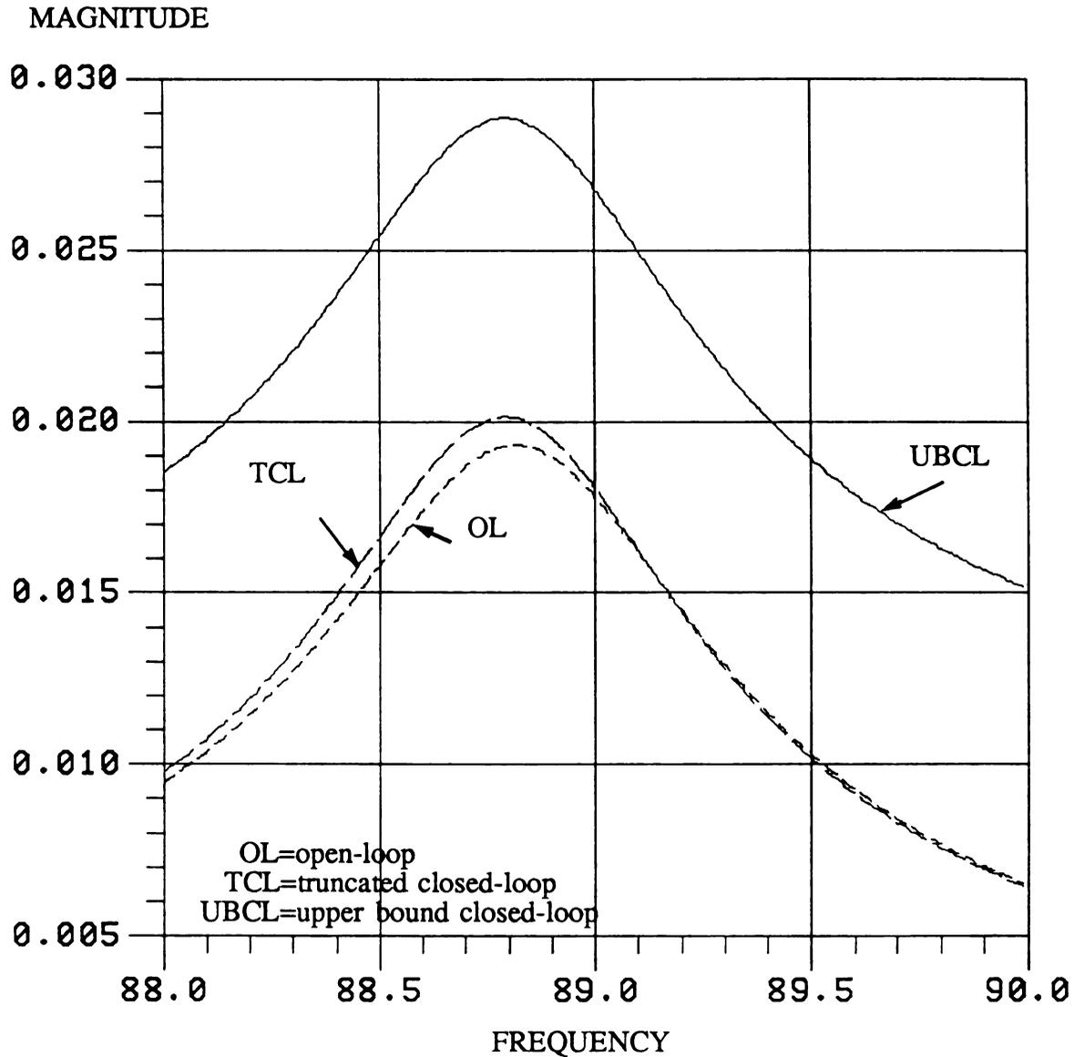
Figure 5.8: Detailed closed-loop frequency response of the 3rd mode
