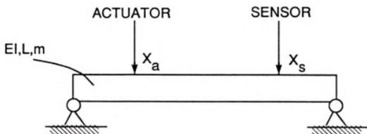
Figure 4.3: The Bernoulli-Euler beam showing the actuator and sensor
