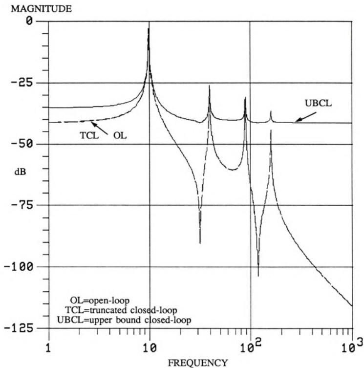
Figure 5.5: Closed-loop frequency response for the system in Fig. 5.2
