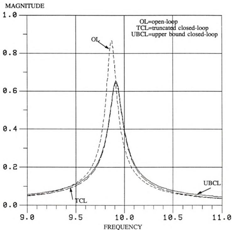
Figure 5.6: Detailed closed-loop frequency response of the 1st mode
