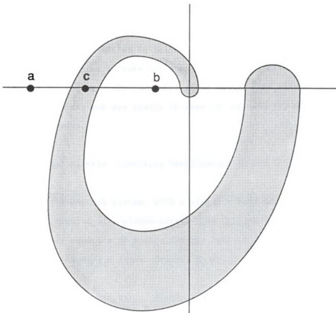
Figure 4.2: The different stability cases of the modified Nyquist criterion - a) guaranteed stability, b) guaranteed instability, and c) undetermined stability
