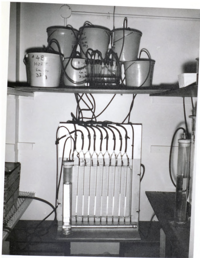
Fig. 1. Apparatus for measuring CO 2 production of potato tubers.
