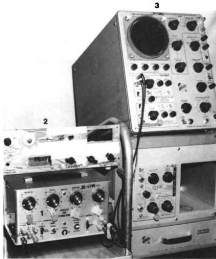
Fig. 4.11. Grass Stimulator (1), auxiliary stimulator (2) and Tektronix Oscilloscope (3). The auxiliary stimulator provided alternating square pulses of sufficient current level to create tetanic forces in the muscle. The Grass Stimulator was used to vary the frequency and time duration of the pulses and the oscilloscope allowed for initial calibration of the stimulator circuit.
