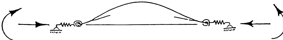
Figure 2.24 Idealization of The Steel Struts End Connections by Linear and Rotational Springs
