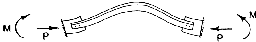
Figure 2.19 Bending Moment in Connections Caused by Bowing of Steel Struts
