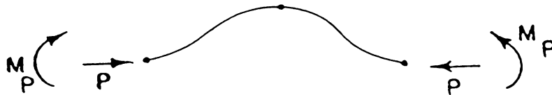
Figure 2.20 Formation of End Plastic Hinges Due to The Flexural Yielding of Connections
