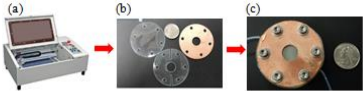
Figure 19. (a) CO 2 laser cutter (b) Upper left: filter piece, upper right: holder, low center: spacer (c) Final assembled PC sensor including the capillary inlet and outlet of samples
