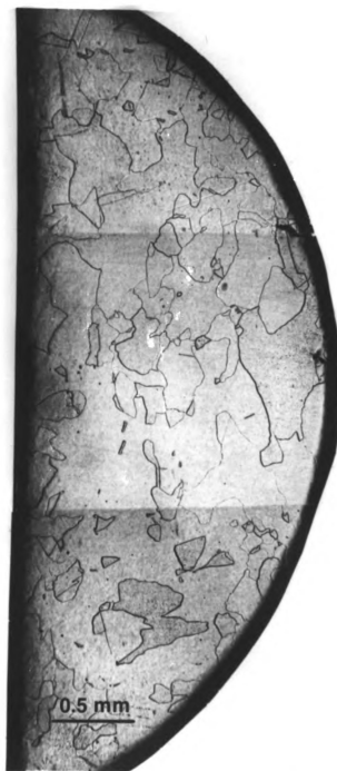
Fig. 4-16. The microstructure in a plane perpendicular to the loading direction and containing the smallest diameter region of an hour-glass shape Ni fatigued at 600°C with 1% total axial strain amplitude.
