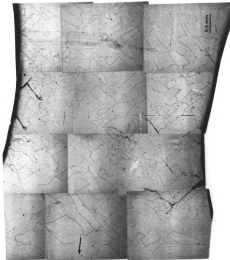
Fig. 4-17. The microstructure in a plane parallel to the loading direction of an hour-glass shape Ni fatigued at 600°C with 0.3% total axial strain amplitude.
