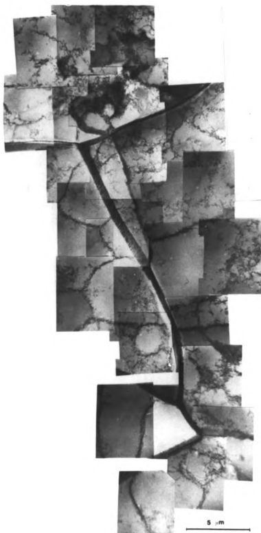
Fig. 4-31. Dislocation structure around a grain boundary of a Ni tested at 600°C with 1.7% total strain amplitude.
