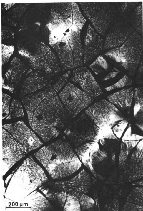
Figure 34. Network of inter-spherulitic boundaries in a completely devitrified 70-30-0, 5 glass. The arrows indicate the boundary network.
