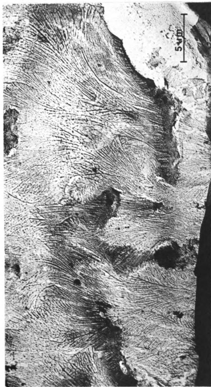
Figure 30. Electron micrograph of fibrous growth morphology in spherulites grown at 400°C in 70-30-0.5 glass.
