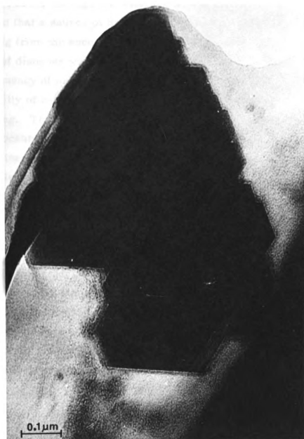
Figure 36. Electron micrograph of faceted crystal growth in a 60-40-0.1 glass after devitrification at 450°C for 1 hour.
