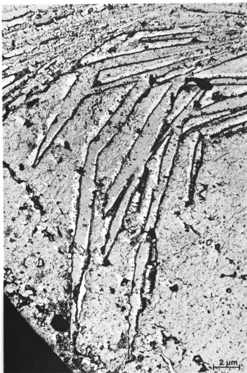
Figure 32. Electron micrograph of branching fibers in a spherulite grown at 550°C.
