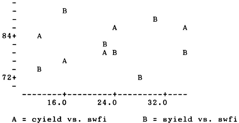
Figure D22. Scatter plot of relative corn yield (cyield,%,A) and relative soybean yield (syield,%,B) vs. the water table fluctuation wety stress index (swfi,m\*hr/hr) for the 1987 growing season at the Bannister site.
