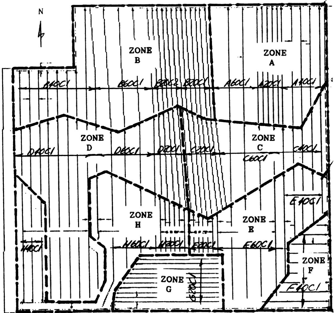
Figure 3. Bannister site water management zones (A through H), subsurface drainage pipe layout (lateral spacing 6, 12, 18 m) and treatments within each zone (for example A40C1).
