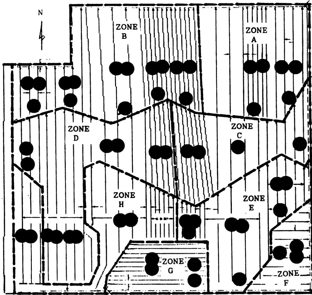
Figure 6. Bannister site well locations. Groups of three within a set of laterals equally spaced are located 1 m from the lateral, midway between the laterals and at the upper end of the water management zone, midway between laterals.
