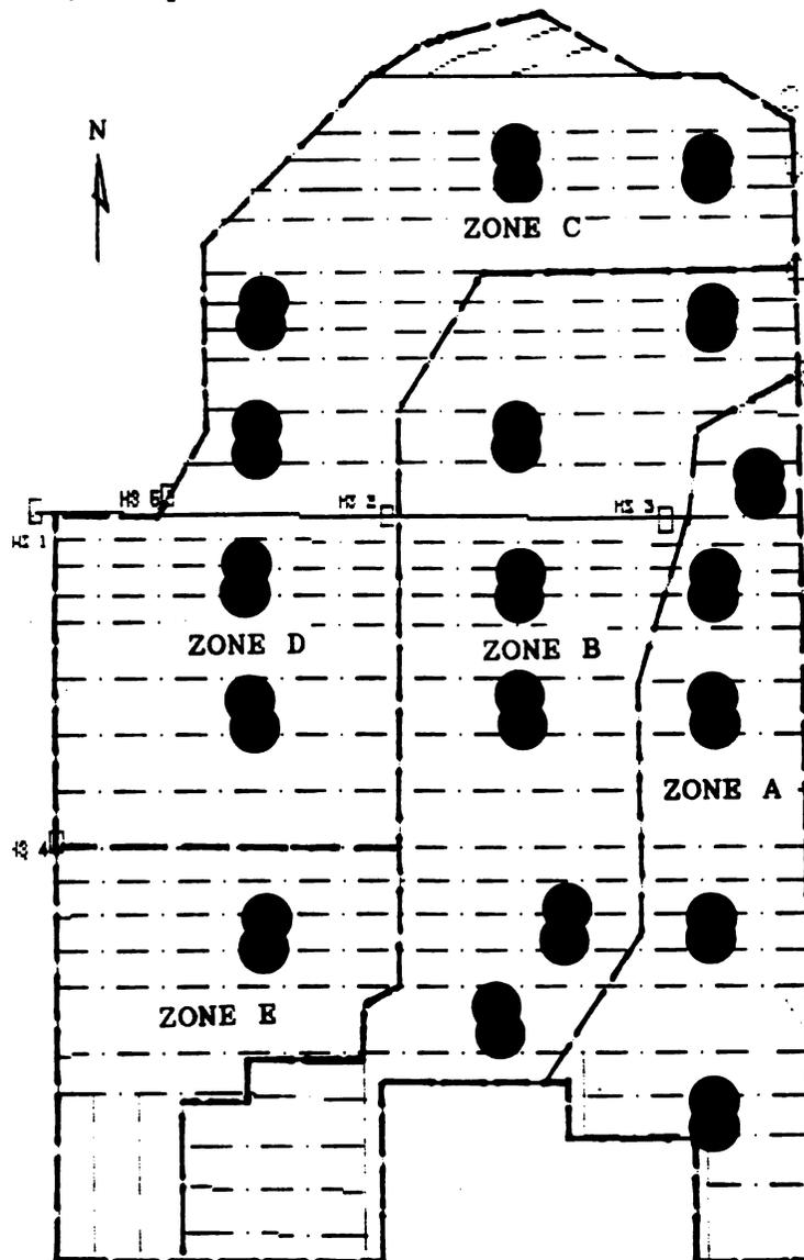
Figure 7. St. Johns site well locations. Groups of two within a set of laterals equally spaced are located at 1 m from the lateral, midway between the laterals and at the upper end of the water management zone, midway between laterals.
