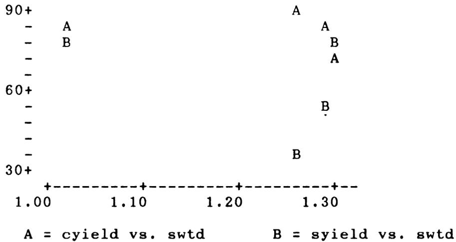
Figure D34. Scatter plot of relative corn yield (cyield,%,A) and relative soybean yield (syield,%,B) vs. mean depth to the water table (swtd,m) during the 1987 growing season at the St. Johns site.
