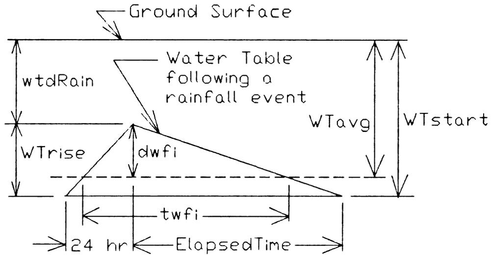
Figure 20. Schematic of assumed water table elevation vs. time following a rainfall event.
