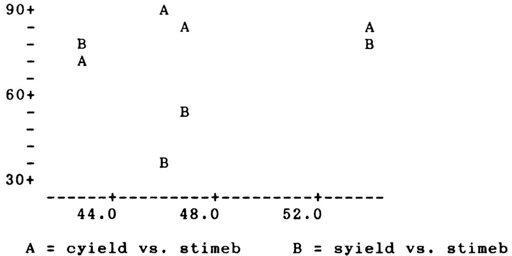
Figure D35. Scatter plot of relative corn yield (cyield,%,A) and relative soybean yield (syield,%,B) vs. time water table was below the mean water table depth (stimeb,%) during the 1987 growing season at the St. Johns site.
