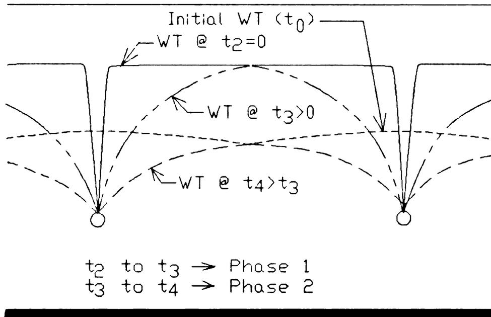
Figure 19. Schematic showing change in water table (WT) with time (t) following a rainfall event through water table drawdown with the subirrigation system initially in a subirrigation mode.
