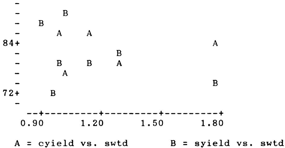
Figure D18. Scatter plot of relative corn yield (cyield,%,A) and relative soybean yield (syield,%,B) vs. mean depth to the water table (swtd,m) during the 1987 growing season at the Bannister site.
