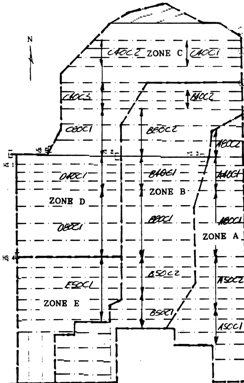
Figure 5. St. Johns site water management zones (A through E), subsurface drainage pipe layout (lateral spacing 12, 17, 24 m) and treatments within each zone (for example A50C1).
