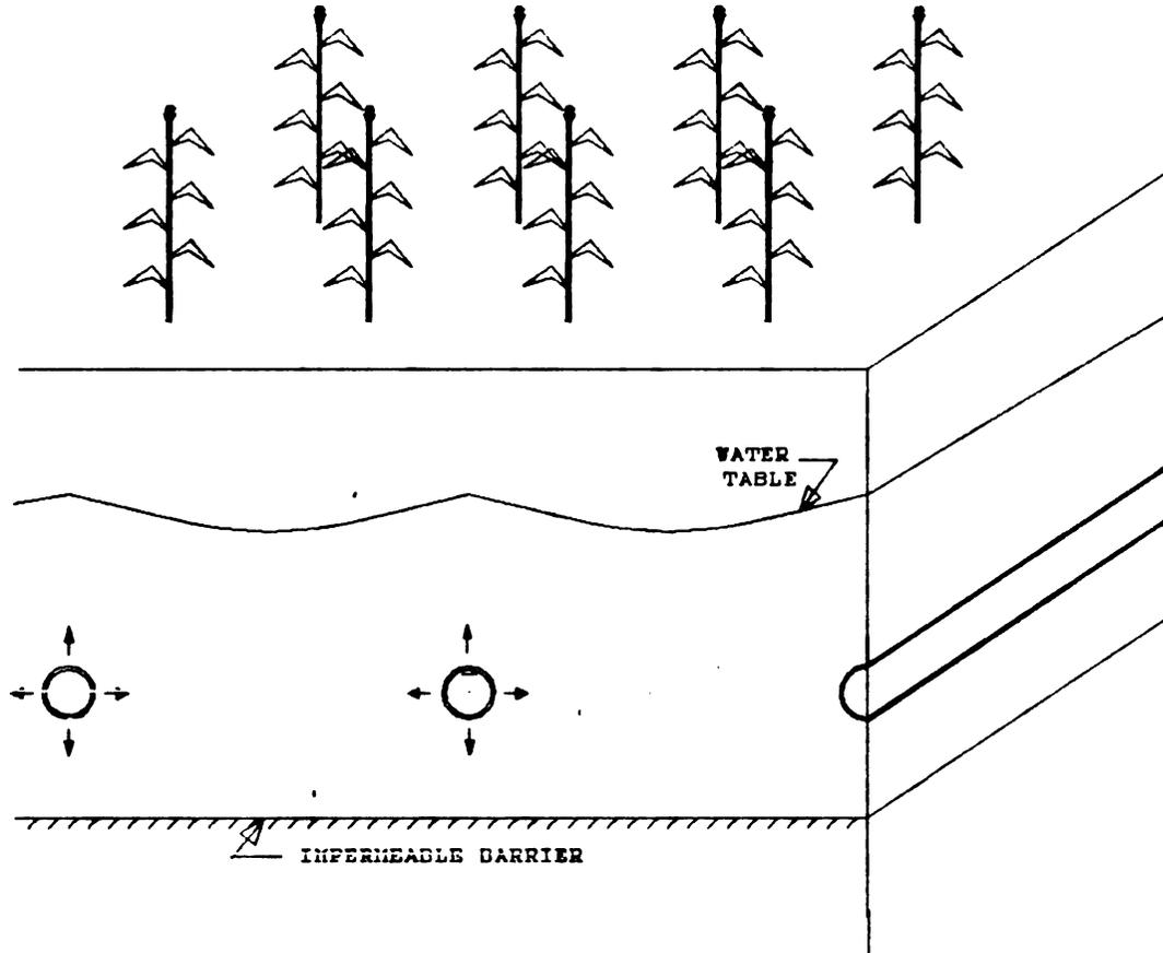
Figure 1. Cross sectional schematic of a water table management system operating in a subirrigation mode.
