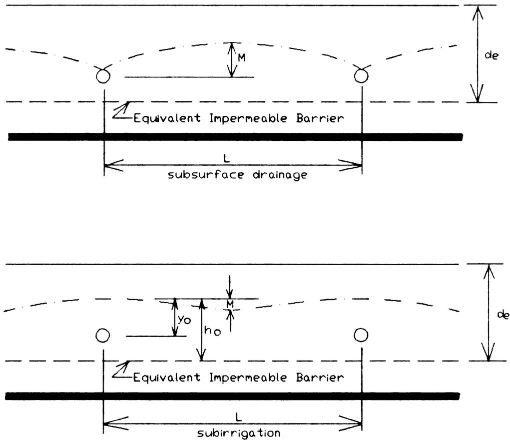
Figure 18. Subsurface drainage/subirrigation lateral spacing design notation.
