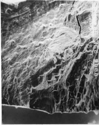
Fig.16 : Fracture Surface of Unmodified DS-Nickel, Showing the Profusion of Micro-cracks in the Matrix
