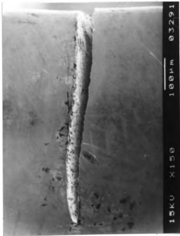
Fig. 15 : Fatigue Crack Initiated at the Edges of Surface Modified DS-Nickel Specimens
