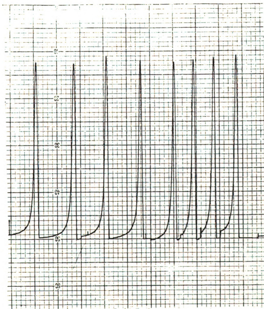
Figure 4-22: 8 injections of a 0.08 mM solution \text{H}_2\text{O}_2 using Patton's detector. The RSD of the measured absorbance is 1.95%.
