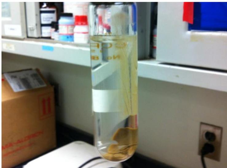
**Figure 4.4** Separation aqueous phase from soil after centrifuge
