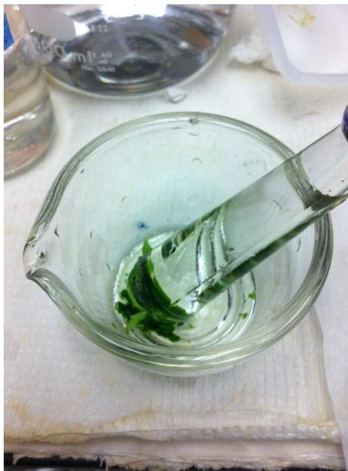
**Figure 5.11** Plant parts maceration by pestle and mortar
