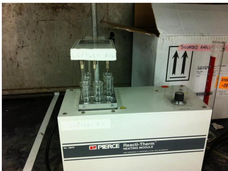
**Figure 6.2** The condensation of collected root exudates by evaporation unit
