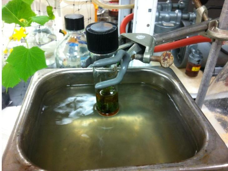
**Figure 5.12** Plant extracted by sonication in ultrasonic bath
