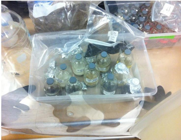
**Figure 6.5** The set of bottles prepared in glove box under N<sub>2</sub> atmosphere
