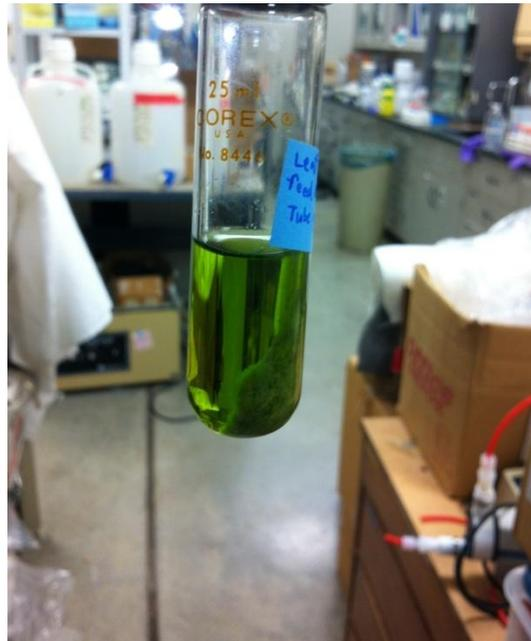
**Figure 5.13** Supernatant separation from plant tissue after centrifuge
