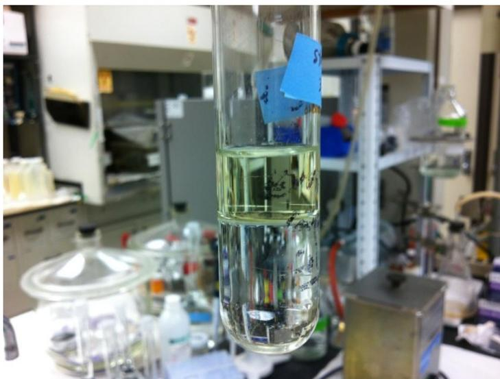
**Figure 2.4** Octanol and aqueous phase separation in shake flask experiment (For the interpretation of the references to color in this and all other figures, the reader is referred to the electronic version of this dissertation)
