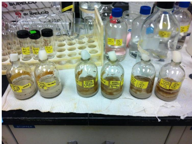
**Figure 6.4** The prepared bottles for decomposition of *A. Clematitis* seeds in aerobic condition
