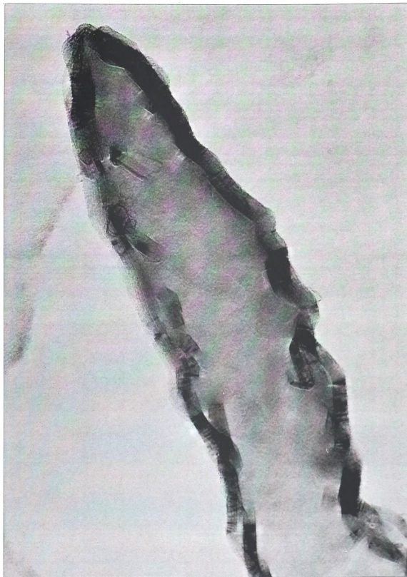
FIGURE 34c. CDA50 TEM picture ( 3 \times 190,000 : 1 \text{ cm} = 175 \text{ \AA} )
