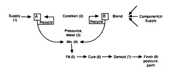
FIGURE 1.2 The Eight Unit Operations for RIM
