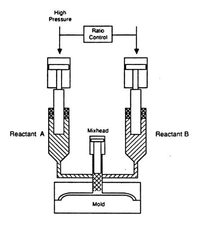
FIGURE 1.1 Schematic of a RIM Machine
