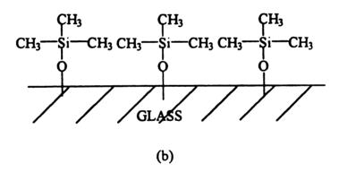
FIGURE 5.7 Idealized Monolayer of Condensed (a) Methyltrimethoxysilane (b) Trimethylchlorosilane on Glass Surface
