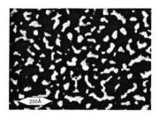
FIGURE 2.3 A Transmission Electron Micrograph of a Segmented Polyurethane
