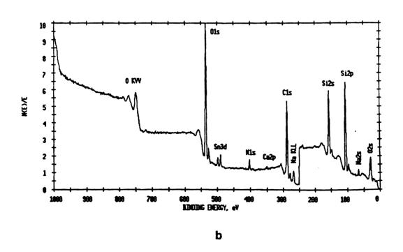
FIGURE 4.7 XPS Survey Scans (a) Bare Soda-Lime Glass, (b) Failed Glass Sample 10B
