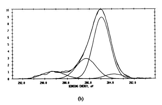
FIGURE 5.6 Curve Fitted C 1s Spectra of Failed Glass Surfaces Taken at 15° Photoelectron Take-Off Angle (a) Sample 1D (b) Sample 1D with BDO Coated Glass
