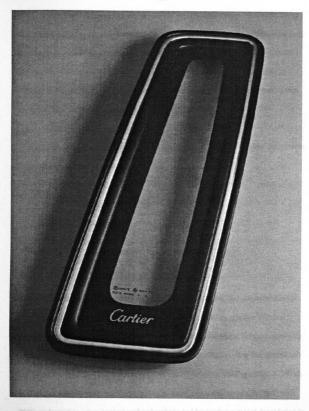
FIGURE 1.8 An Encapsulated Modular Window
