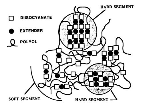
FIGURE 1.3 Schematic Representation of Phase Separation in Polyurethane Segmented Block Copolymers
