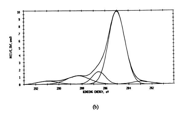
FIGURE 5.10 Curve Fitted C 1s Spectra of (a) Control Glass Sample (b) Glass Treated with BDO and Rinsed
