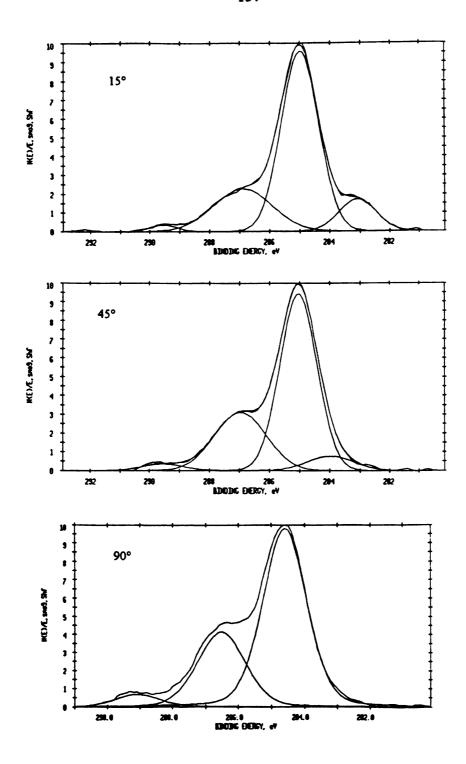
FIGURE 5.9 Curve Fitted C 1s Spectra of Adhesion Failed 10D Glass Samples Precoated with Methyltrimethoxysilane Taken at 15°, 45°, and 90° Photoelectron Take-Off Angles
