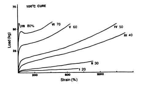
FIGURE 1.7 Load vs. Strain for Polyurethanes at Various % Hard Segment Content
