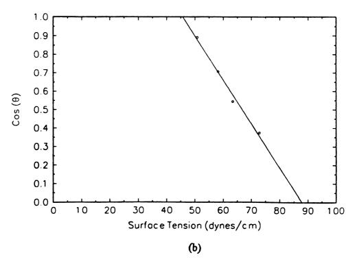
FIGURE 5.1 Zisman Plots of (a) 1C Polyurethane Sample with 46.7 wt. % Hard Segment and (b) HS Polyurethane Sample with 100% Hard Segment
