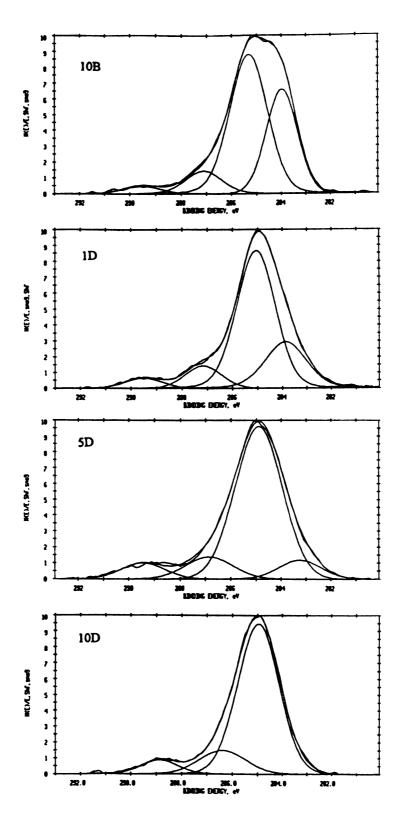
FIGURE 4.8 Curve Fit C 1s Spectra of Failed Glass Samples at 90° Photoelectron Take-Off Angle
