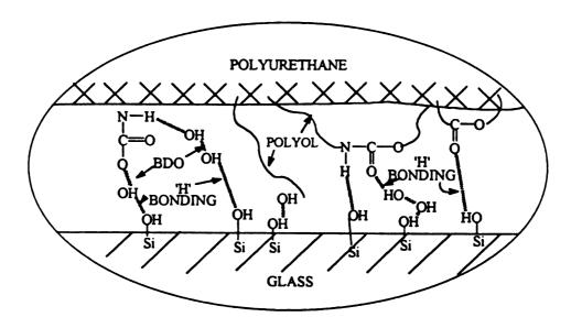
FIGURE 5.11 Schematic of Polyurethane/Glass Interphase Region with Probable Hydrogen Bonding Mechanisms
