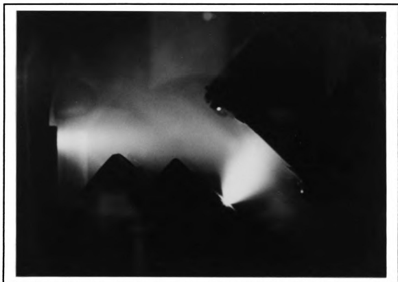
Figure 36. Laser induced plume and oxygen ion-beam
