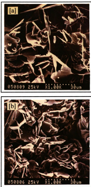
Figure 45. Scanning electron micrographs of (a) 90 Watts laser-processed sample, sample A, and (b) conventionally processed sample, sample C
