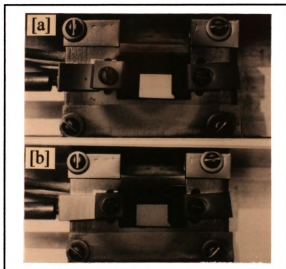
Figure 51. Silver substrates in substrate heater after laser vapor deposition with 0.25 ms laser pulses, 40 \text{ J/cm}^2 pulse energy density and 100 mtorr of \text{O}_2 deposited (a) without ion-beam and (b) with ion-beam
