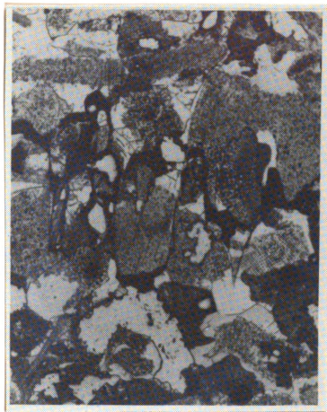
Figure 7a: Cementation was essentially complete before development of pressure solution features. Note type 1A pressure solution feature cutting both allochem and cement, and note cement supporting allochem undergoing dissolution. 45X scale = 100 \mu
