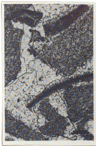
Figure 2: Dominant syntaxial overgrowth cements on crinoid fragments and minor sparry cement on brachiopods. 80X scale = 150 \mu
