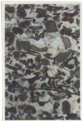
Figure 6: Syntaxial cement on echinoderm fragments. Note dominance of this type of cement over sparry cements developed on multi-crystalline substrates. Typical of clean crinoidal grainstones. 20X scale = 500 \mu
