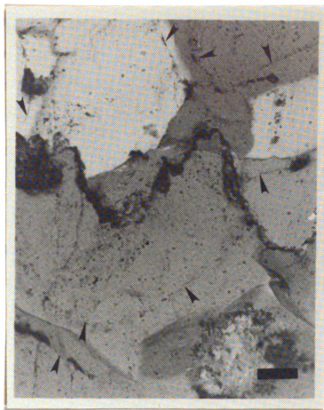
Figure 10: Type 1A stylolite in the Tuscarora sandstone. Note cementation by well-developed quartz overgrowths. Arrows point to dust rings on detrital grains. This sample is texturally analogous to well-cemented grainstones in the Alpena limestone. 240X scale = 50 \mu
