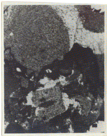
Figure 7b: Note pressure solution removing both cement and allochem in this photograph. 150X scale = 30\mu
