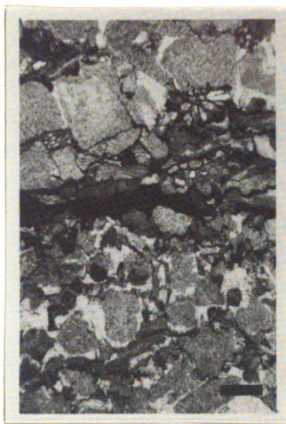
Figure 7c: Note pressure solution removing both cement and allochem in this photograph. Note fitted fabric texture developed above and beneath central pressure solution feature. Pressure solution of a distinctly different style than Figures 7a and 7b. 25X scale = 500 \mu
