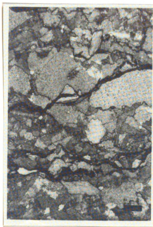
Figure 8: Pressure solution in fitted fabric texture. Note lack of apparent reprecipitation of dissolved carbonate. 20X scale = 500 \mu
