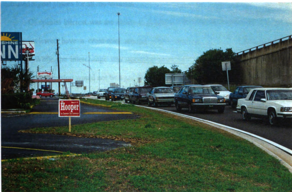
Figure 5.4: Dual left-turning traffic is backing up, blocking right-turning traffic.
