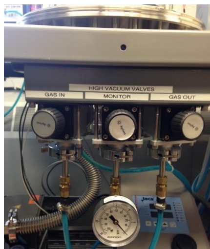
Figure B.18. High vacuum valves below the furnace. The gas in and gas out valves should be closed before pumping down the bell jar chamber.
