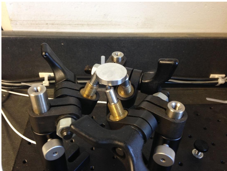
Figure 2.1. Typical setup of tripod arrangement of RUS transducers, with specimen on top and the transducer tips near the edge of the specimen.
