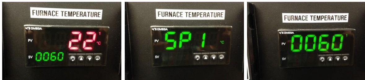
Figure B.21. Furnace temperature controller, from left, in run mode, selecting set point 1, and setting set point 1 to 60°C.
