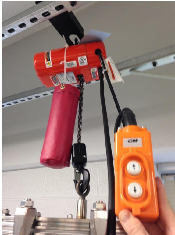
Figure B.16. Hoist and controls to operate up and down. Note the hoist is mounted to a rail for movement left and right, and that the chain has some slack when the bell jar is in position.
