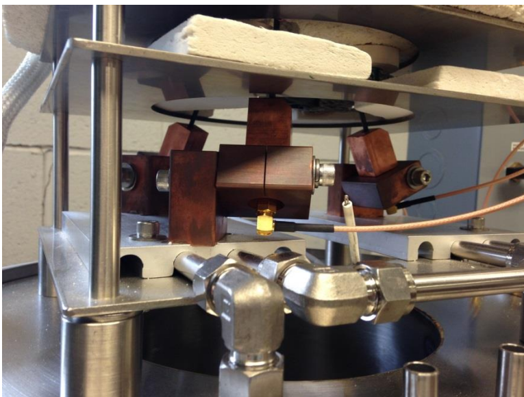
Figure B.9. The three transducers are mounted to copper blocks on the chiller plates underneath the furnace. The mount swivels to allow the angle of the transducer to be adjusted.
