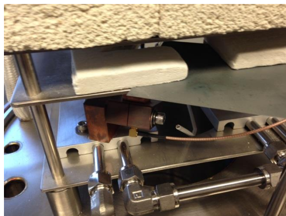
Figure B.11. Molybdenum baffle being inserted around buffer rods.
