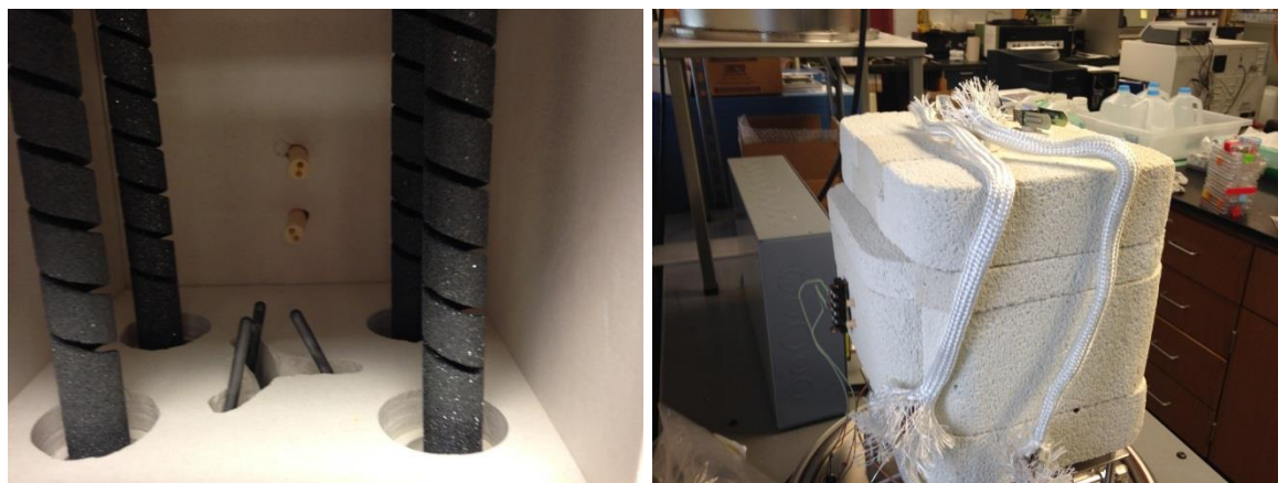
Figure B.27. The spiral cut hot zone of the heating elements should be completely contained within the furnace. The power connections to the heating elements should be outside the furnace.
