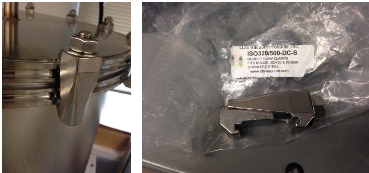
Figure B.17. Clamps for the bell jar. The same clamps are used to secure the top and base of the bell jar.
