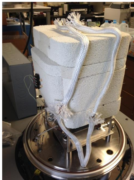
Figure B.3. Braided insulation must be in place around the conductors to the heating elements to prevent a short.
