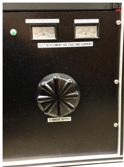
Figure B.24. Heater ammeter, heater voltmeter, and variac output knob on control box.
