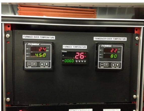
Figure B.20. From left, the furnace over temperature limit controller, furnace temperature controller, and the transducer over temperature limit controller.
