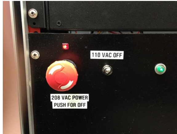
Figure B.22. 208 VAC power switch with red indicator light on, and 110 VAC power switch with green indicator on.
