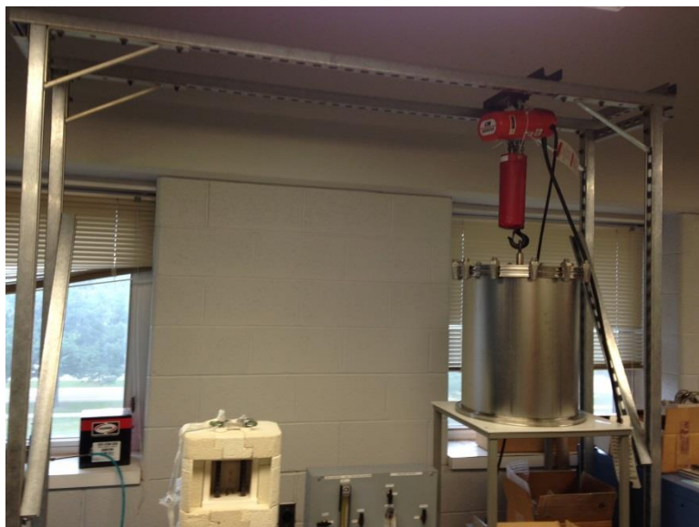
Figure B.25. Bell jar at rest on side table and furnace opened. There should be some slack in the chain, allowing all the weight of the bell jar to rest on the table.
