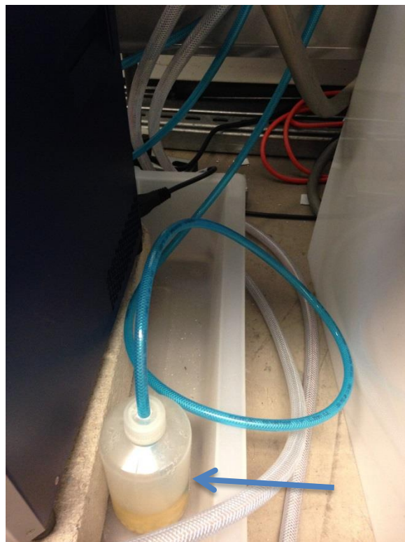
Figure B.7. The bubbler (arrow), with the hose extending out, should be filled to cover the end of the hose with liquid to prevent air from entering the hose.
