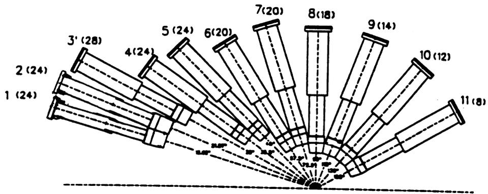
Figure 2.6 Half-plane section of the upgraded Miniball/Miniwall array. The rings of the Miniwall are labeled with 1-2 and rings 3'-11 label the individual rings for Miniball. The number of detectors per ring are given in parentheses. The polar angles for the centers of detectors are indicated. The dashed horizontal line indicates the beam axis.
