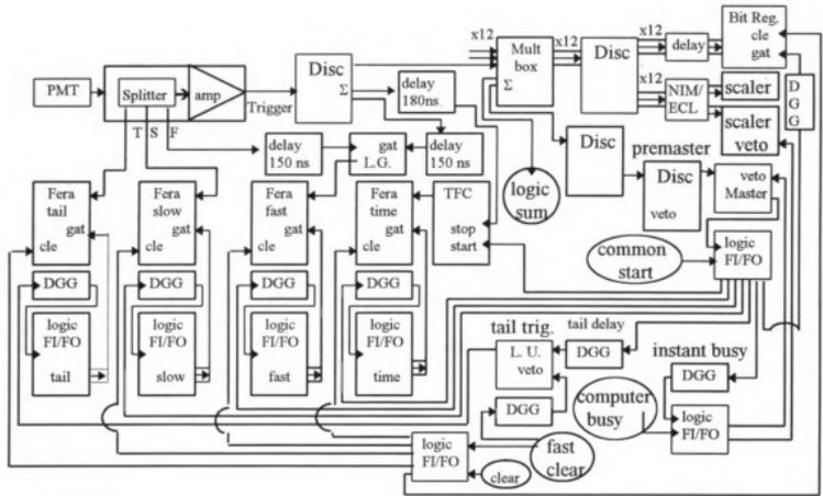
Figure 2.10 Schematic electronics diagram of the data acquisition of the electronics for the Miniball array alone. The Disc, Split., DGG, Fera, Amp., L.U. and FI/FO present Discriminator, splitter, delay and gate generator, Fera ADC, amplifier, logical unit and the fan in/fan out models respectively.
