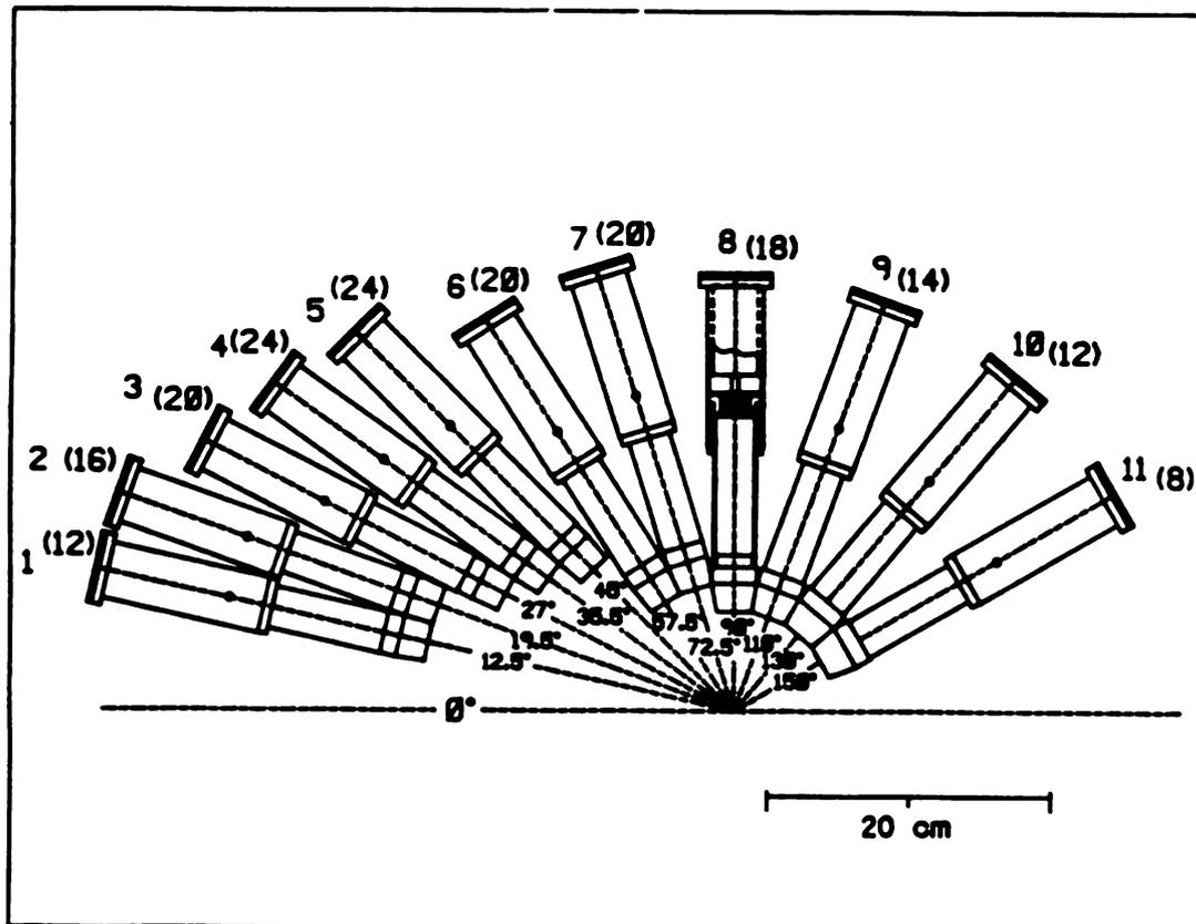
Figure 2.2 Half-plane section of the original Miniball array. Number of detectors per ring are given in parentheses. The polar angles for the centers of detectors are indicated. The dashed horizontal line indicates the beam axis.
