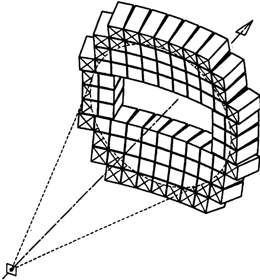
Figure 2.9 Three dimensional geometric diagram of the Catania hodoscope array.
