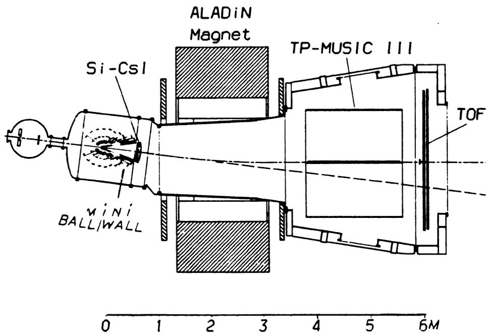
Figure 2.1 The schematic drawing of the experimental set-up. This experimental apparatus includes the Miniball/Miniwall array, the Catania Si-CsI hodoscope array and the Aladin spectrometer. The TP-MUSIC chamber and TOF wall are two main components of the Aladin spectrometer.
