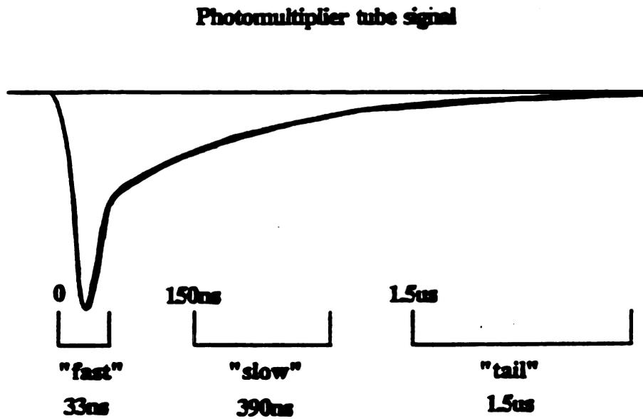
Figure 2.5 Timing and widths of the fast, slow and tail gates.
