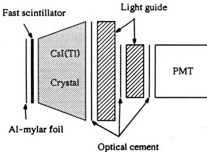
Figure 2.3 Schematic diagram of individual detector elements.
