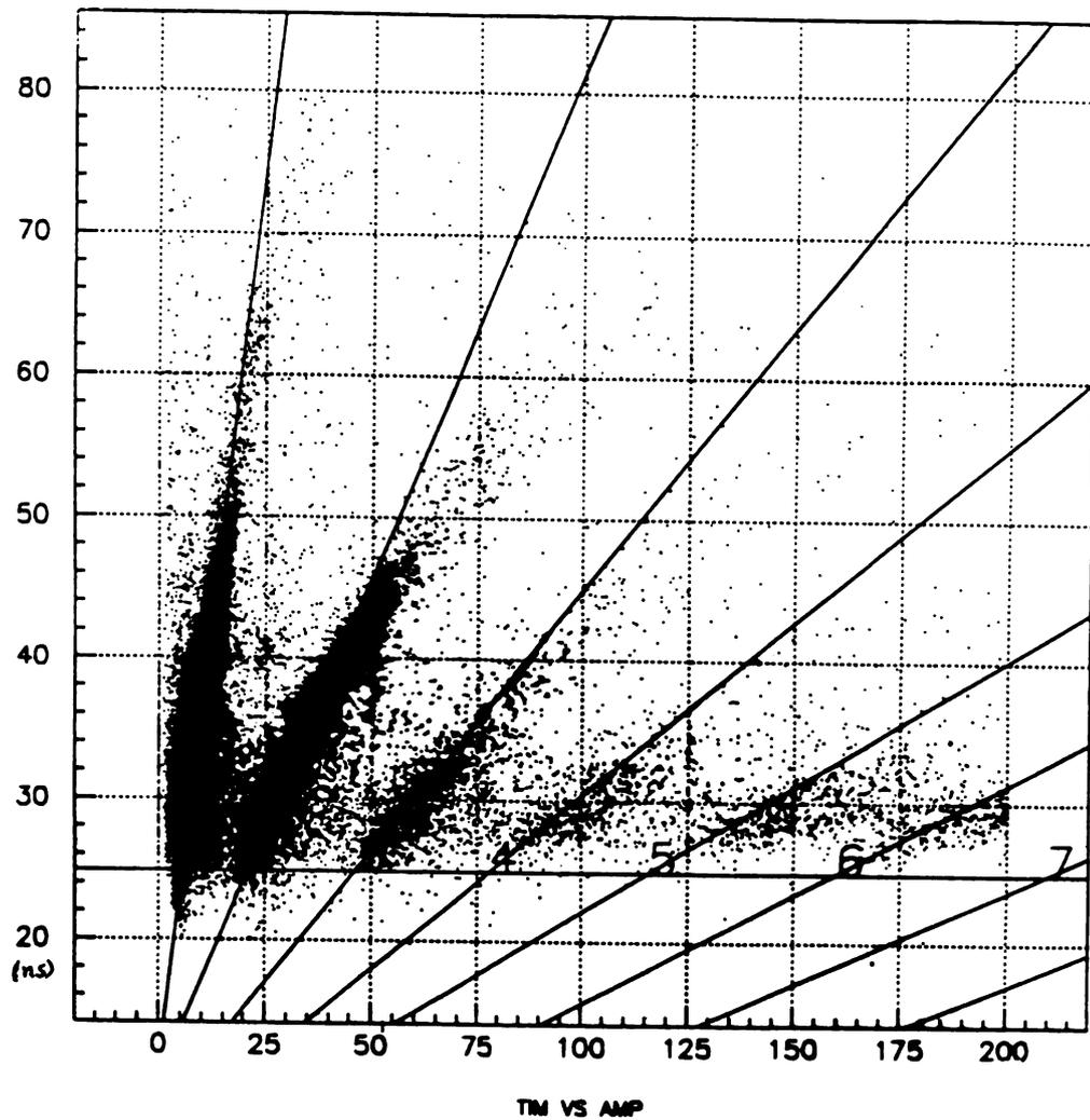
Figure 3.11 The flight time is plotted versus the light output of particles detected in the front 100 scintillators of the ToF wall which are used for the particle identification. The charge lines are indicated by the straight lines.
