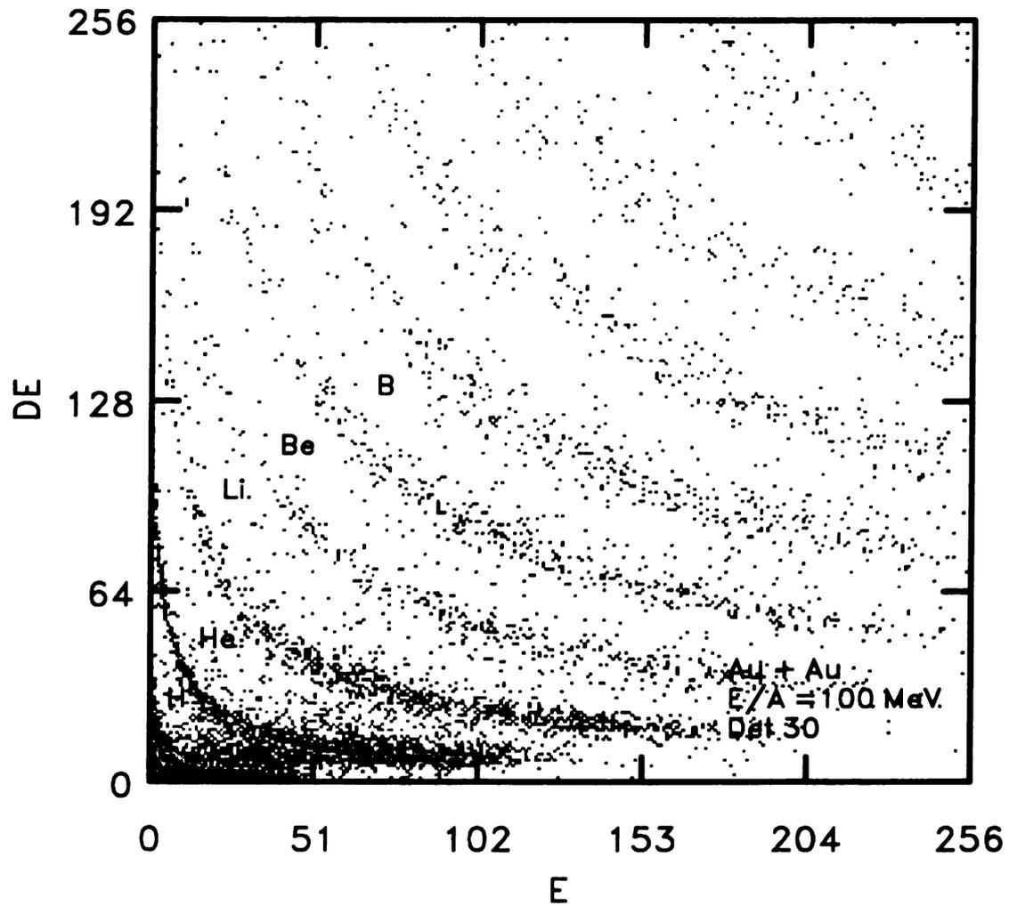
Figure 3.9 DE (signal of Si) versus E (signal of CsI) for the Catania hodoscope is plotted for detector 30 at  $E/A = 100$  MeV collisions.
