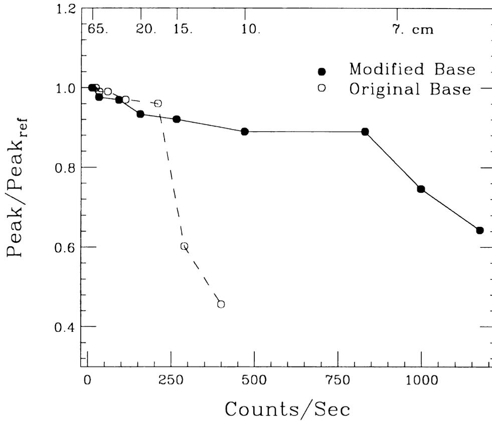
Figure 2.8 The relative magnitudes of the  $\gamma$ -ray peaks are plotted as a function of the counting rate for the two different voltage dividers. The distance between the source and detector is indicated at the top of this Figure.
