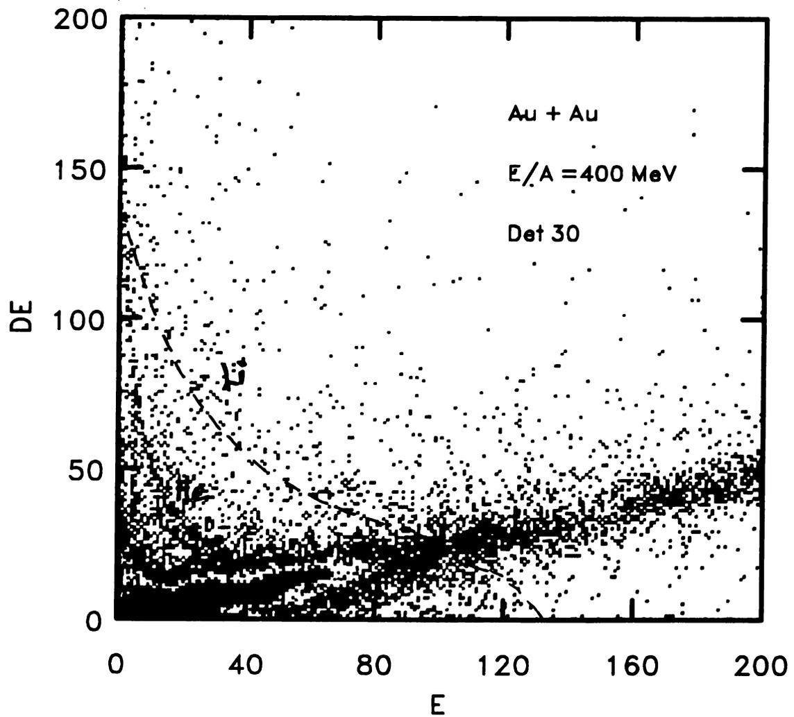
Figure 3.10 DE (signal of Si) versus E (signal of CsI) for the Catania hodoscope is plotted for detector 30 at  $E/A = 400$  MeV collisions.
