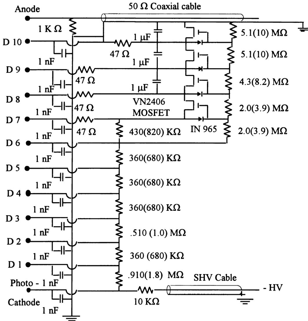
Figure 2.4 Schematic diagram of the upgraded active voltage divider used for Rings 9, 10 and 11 of the Miniball array. The value of resistors for the original divider are listed in parenthesis.
