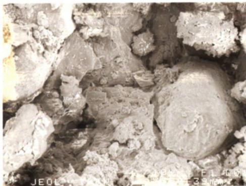
SEM photograph showing halite efflorescence (a) growing between sand grains (b) at Morrill Hall. The halite is pushing the grains apart.
