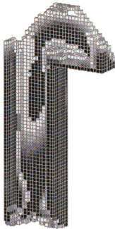
Figure 4.38: Anti-symmetric tower example standard solution. (Front half of structure removed)
