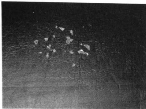
**Figure 4.9 Progeny PET Particles from Single Particle Impact at 92.3 m/s and 22°C:
