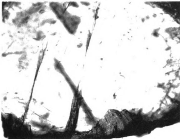
**Figure 4.11** Optical Microscopy Photograph of PVC Particle Ground at 92.3 m/s and 0°C
