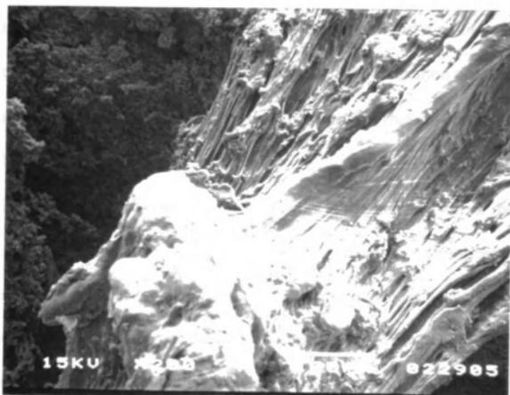
Figure 3.12 SEM of PVC Ballistics Sample Impacted at 398 m/s
