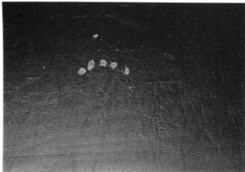
**Figure 4.5** Progeny PVC Particles from Single Particle Impact at 53.3 m/s and 22°C:
