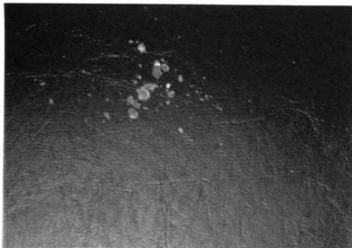
**Figure 4.6** Progeny PVC Particles from Single Particle Impact at 92.3 m/s and 22°C:
