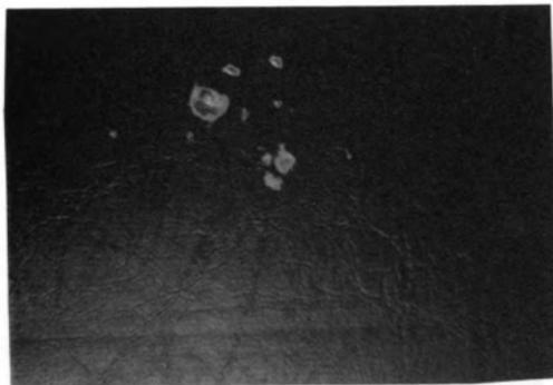
**Figure 4.8 Progeny PET Particles from Single Particle Impact at 53.3 m/s and 22°C:
