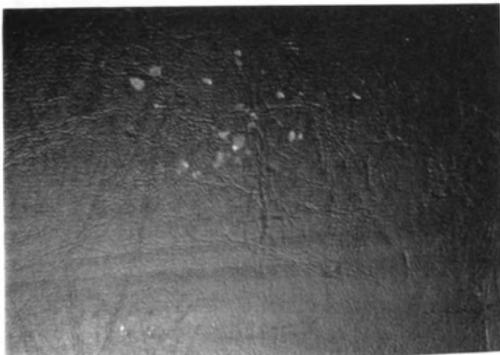
**Figure 4.7 Progeny PVC Particles from Single Particle Impact at 92.3 m/s and 0°C
