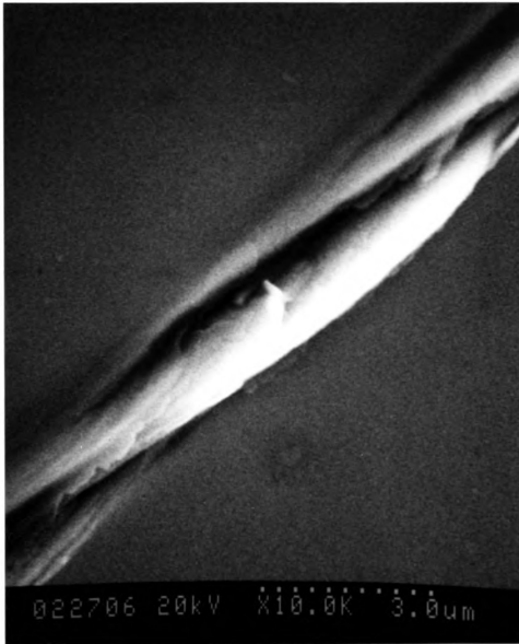
Figure 4-33. Persistent slip band structure in bare copper after 500 cycles ( 2\Sigma\Delta\epsilon_p = 2 ).
