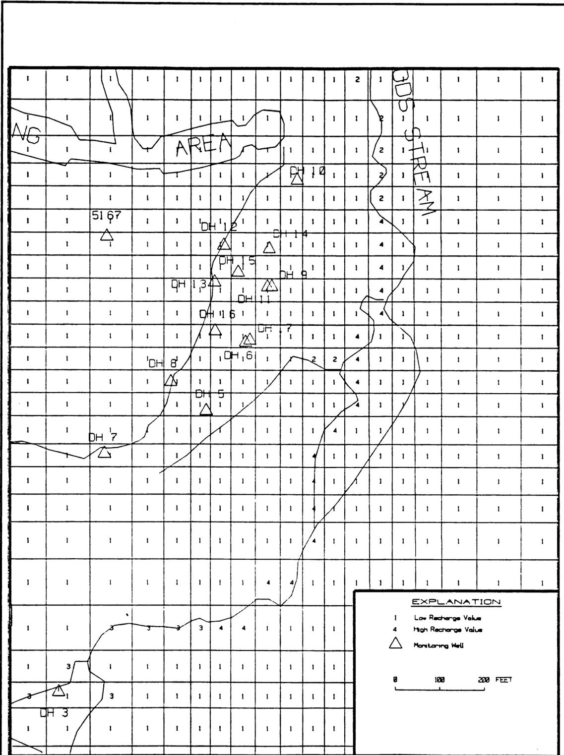
Figure 14: Recharge Node Values For Groundwater Flow Model
