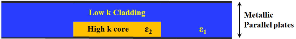
Figure 2.34 Schematic of waveguide with high- k core surrounded by low- k material in metallic parallel plates.
