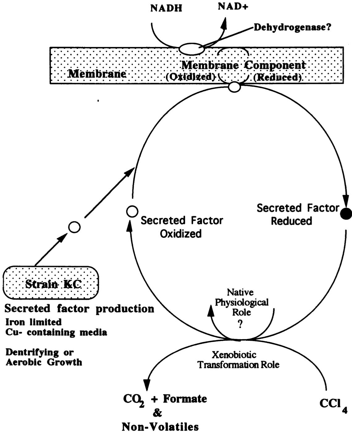
Figure 7.1 Model of proposed  $\text{CCl}_4$  transformation process by *P. stutzeri* KC.
