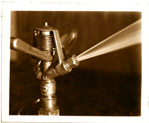
Fig. 36. Jet of water issuing from a quatrefoil orifice at 40 psi.
