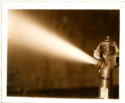
Fig. 12. Jet of water issuing at 40 psi from a \frac{1}{4} inch diameter circular orifice (using sprinkler with \frac{1}{2} inch riser connection).
