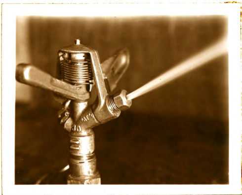
Fig. 35. Jet of water issuing from a square orifice at 40 psi.
