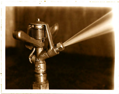
Fig. 28. Jet of water issuing from an equilateral triangular orifice at 40 psi.
