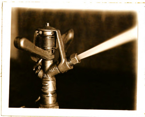
Fig. 23. Jet of water issuing from a 1/4 inch diameter circular orifice, pressure 40 psi (using sprinkler with 3/4 inch riser connection).
