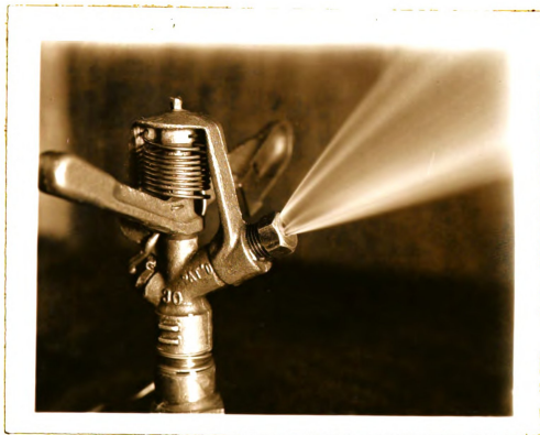
Fig. 30. Jet of water issuing at 40 psi from an isosceles triangular orifice with an abrupt entrance into the orifice.
