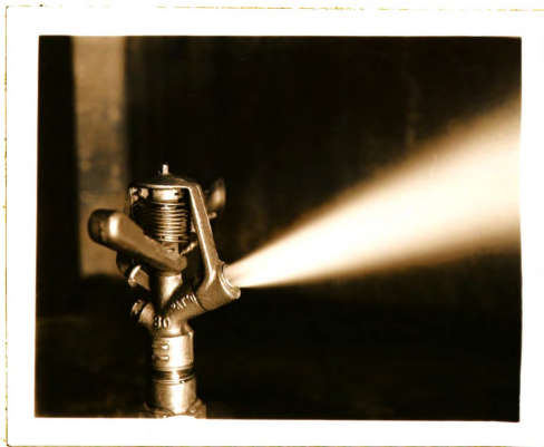
Fig. 39. Sprinkler with 7/16 inch diameter tube cut off at body of sprinkler operating at 40 psi.
