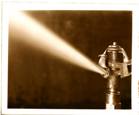
Fig. 44. Jet of water issuing at 40 psi from a 5/32 inch diameter tube soldered into the sprinkler body.
