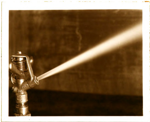
Fig. 20. Jet of water issuing at 40 psi from a \frac{1}{4} inch diameter circular orifice with cylindrical portion of nozzle removed at the end of the taper section.
