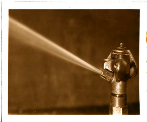
Fig. 37. Jet of water issuing at 40 psi from the nozzle with a side slot.
