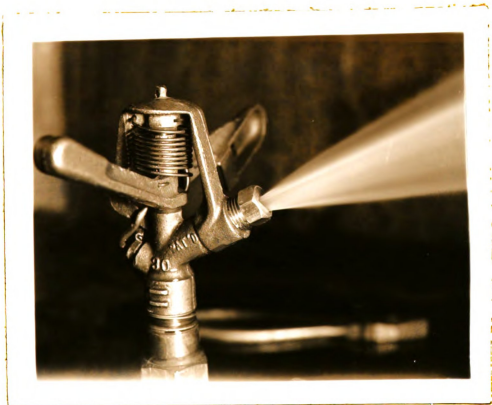
Fig. 29. Jet of water issuing at 40 psi from an isosceles triangular orifice with one vertex rounded.
