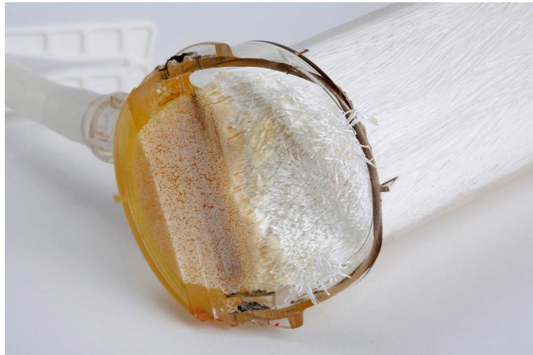
**Figure 3.3 Hollow Fiber Chamber Reactor Cross Section Schematic and Image.** Schematic of HFCR cross section (Top) showing diffusion action of nutrients and drug from the capillaries to the extra capillary space, with the simultaneous removal of waste. An image of a open HFCR cartridge showing porous capillaries (Bottom). Image reproduced with permission from Fiber Cell Systems.
