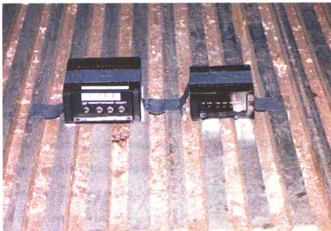
Figure 8: Mounted EDRs on the empty truck floor
